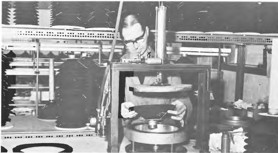
A vital part of the speaker manufacturing process. A cone is mated with its surround of Flexiprene synthetic elastomer.
