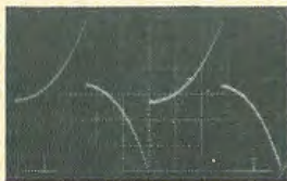
Square-wave response to 50 Hz, left, and to 10 kHz, right.
