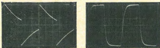
Square-wave response to 50 Hz, left, and to 10 kHz.
