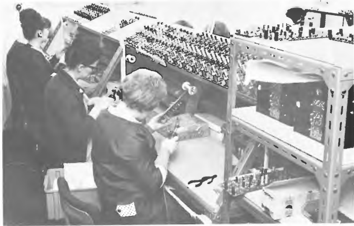
Assembly of components on printed circuit boards for the WHF20 amplifier.
