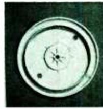
Another important feature is the 50H turntable. It is a heavy, one-piece, non-ferrous metal casting, lathe-turned to precise dimensions and then individually dynamically balanced. This contributes to the smooth, steady motion of the turntable, free of rumble, wow and flutter.
