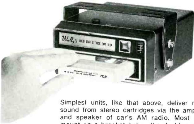
Simplest units, like that above, deliver mono sound from stereo cartridges via the amplifier and speaker of car's AM radio. Most units mount on a bracket below the dashboard. . .
