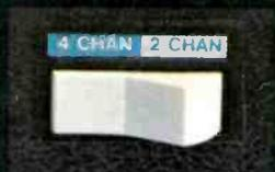
left ear cup. In the 4-channel position, two 1½-inch dynamic driver elements in each ear cup deliver breathtaking quadraphonic sound from either matrix or discrete systems. In the 2-channel position, both drivers in each ear cup are connected in parallel for an unparalleled sound of 2-channel stereo. Either way, the switch to Koss Quadrafones is worth it.
