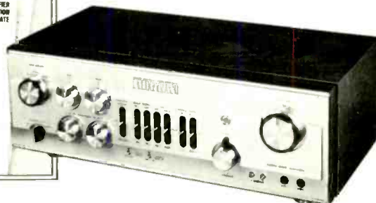
Luxman C-1000 Preamplifier —Total harmonic and intermodulation distortion: 0.007% at 2.5 V, 20 Hz-20 kHz, all output signals. Frequency response: 2 Hz-80 kHz, +0, -0.5 dB. Signal-to-noise: >65 dB. Phono overload: 450 mV @ 1 kHz, 3.5 V @ 20 kHz. RIAA equalization: \pm 0.2 dB. Features include: tape-monitoring and dubbing for two decks, six selectable tone control turnover frequencies, linear equalizer, twin high and low noise filters, variable phono-input impedance, variable input sensitivities, "touch-mute" attenuator, speaker selectors. $895.
