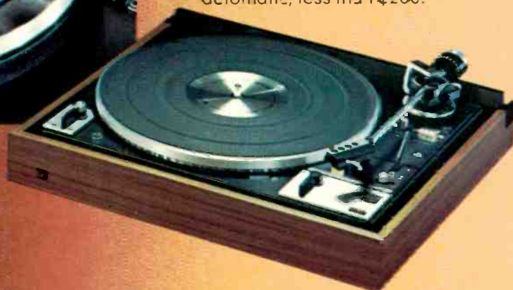
Tonearm of Dual 1249 pivots in four-point gyrosopic gimbal, suspended within a rigid frame. Each gimbal is hand-assembled, and special gauges assure that each will conform to Dual's stringent specifications.
