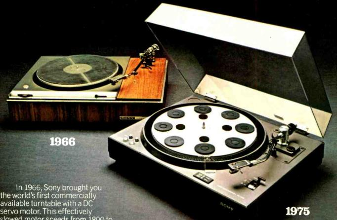
In 1966, Sony brought you the world's first commercially available turntable with a DC servo motor. This effectively slowed motor speeds from 1800 to 300 RPM, producing the lowest rumble figures measured till then. The servo system also drastically reduced wow and flutter, thus giving you a chance to hear what 33-1/3 records sound like at 33-1/3. Quite a revolution.
