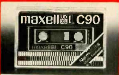
MAXELL UD-XL I CASSETTE. (For "normal" bias and EQ.) New epitaxial cobalt-ferric oxide provides 2.5 dB more sensitivity at all frequencies and 5 to 6 dB more output at high frequencies than conventional tapes. Lowest harmonic and intermodulation distortion.
