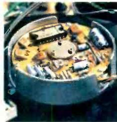
The Garrard DD75 delivers rock-steady speed with a DC motor, governed by an electronic servo system. It is totally immune to fluctuations in household current. The specifications are impressive: rumble -70dB (Din B), wow and flutter 0.03%. The same electronic system provides variable speed control,  $\pm 3\%$ , monitored by an easily-read, illuminated strobe.
