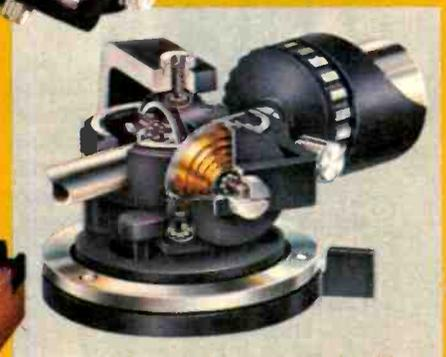
Gimbal-mounted Dual tonearms pivot horizontally and vertically on identical sets of pivot points and high-precision low-friction bearings. Bearing friction: vertical, <math><0.007\text{ gram}</math>; horizontal, <math><0.015\text{ gram}</math>.
