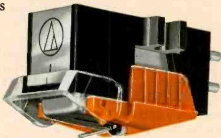
Audio-Technica cartridges have been widely-acclaimed for their great sound, and for good reason. Our unique, patented\* Dual Magnet construction provides a *separate* magnetic system for *each* stereo channel. A concept that insures excellent stereo separation, while lowering magnet mass. And the AT12XE features a tiny 0.3 x 0.7-mil nude-mounted elliptical diamond stylus on a thin-wall cantilever to further reduce moving mass where it counts. Each cartridge is individually
