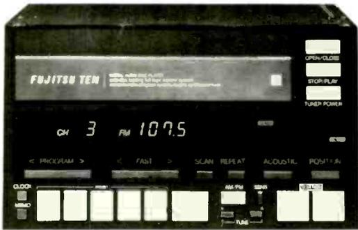
*Most of the prototype car CD players we've seen are dedicated devices—that is, they complement existing car-stereo systems by adding CD playback. This Fujitsu Ten unit goes one better by combining an AM/FM tuner and CD player in one chassis, with some multipurpose controls. And models that add tape playback should appear soon.*
