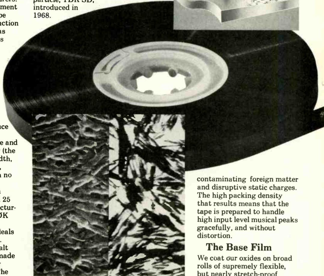
TDK SA tape surface (left) enlarged 30,000 times. TDK Super Avilyn particles (right) enlarged 20,000 times.
