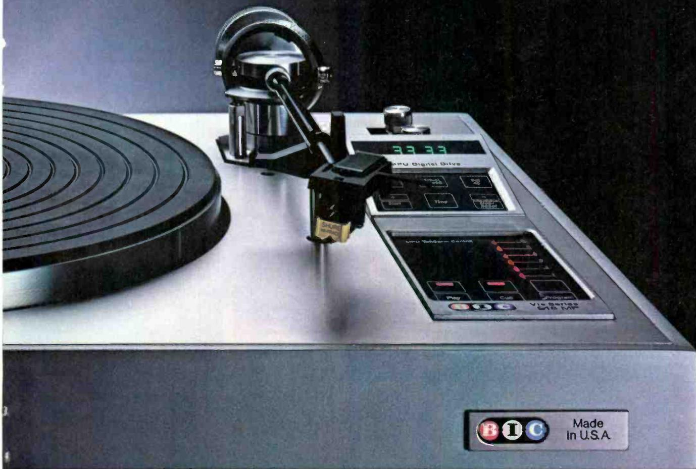
at any price. A digital computer continuously monitors platter speed and corrects variations by means of an AC servo system. Pitch can be varied by 3% up or down and locked in. It's standard on the four top B-I-C models as well as . . . a vacuum fluorescent digital display that reads out measured platter speed to .03% accuracy and updates itself every two seconds, and . . . a digital stop watch for timing selections to tape. This is another
