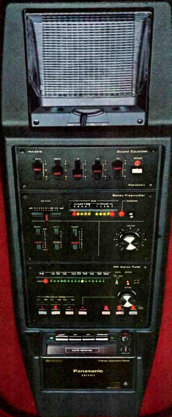
An auto-reverse stereo cassette player with Dolby<sup>®</sup> and CrO<sub>2</sub> tape capability. Plus a preamplifier section that has a special RF amplifier and Double Balance Mixing circuit.
