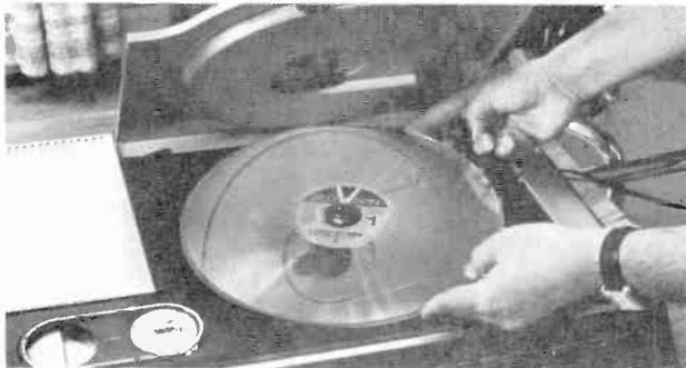
Seat the disc over the spindle, close the lid, and it's movie time. A magnetic interlock, however, prevents the lid from being raised again until the disc has stopped rotating.
