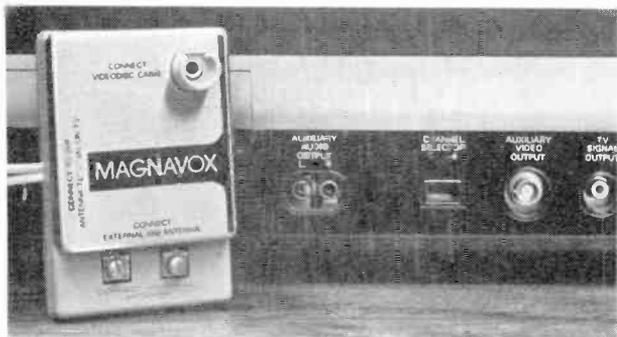
A separate signal-splitting box (left) is necessary to accommodate the Magnavision's output as well as normal antenna or cable-TV feeds. High-quality stereo signals are available via left and right channel audio output jacks.
