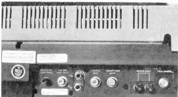
All antenna and cable-TV connections are made directly on the rear of the Laser Disc player, obviating the need for a signal-splitting box. The Laser Disc machine has a PCM adapter output jack for eventual use with a separate digital audio decoder.
