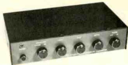
BP Electronics' five-in-one V-1880 processor is among the most versatile video accessories available. It combines a stabilizer to ensure good dubs, an image enhancer to increase detail, an RF converter, a fader, and a dual-output distribution amplifier in one compact box. The V-1880 costs \$250.
