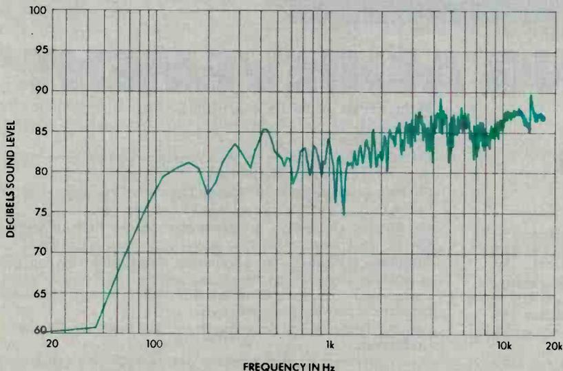
FIGURE 5. WINDOWING REMOVES THE EFFECTS OF ROOM REFLECTIONS FROM THE RESPONSE CURVE AND LEAVES THE AUDIBLY IMPORTANT DETAILS OF THE MEASUREMENT VISIBLE.
