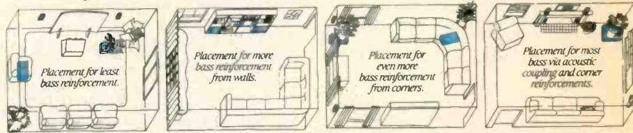
You can put Ensemble's low-frequency units exactly where they should go for superb bass. You can't do this with conventional speakers because you have to be concerned about the upper frequencies coming from the same enclosures as the low ones.
