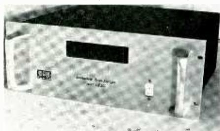
This new amplifier features an ultra fast acting SCR crow bar, FET operational amplifier IC's, thermostatically controlled forced air cooling, over temperature protection, a circuit breaker and plug in circuit modules. The power supply is built around a 2.5KW 35 pound power transformer. The chassis features a welded steel frame for maximum strength and rigidity. The attractive front panel is brushed satin silver with large cast aluminum handles and a hidden display for status indicators.
