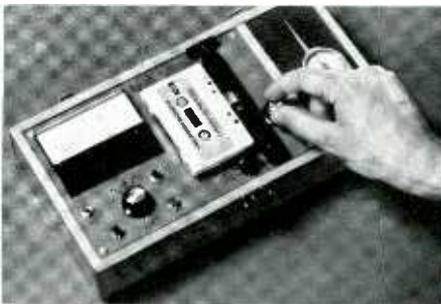
The instrument measures the winding torque in cassettes under varied conditions, and also determines the amount of force exerted on heads by individual pressure pads. The user places a cassette on the instrument's deck, presses the "start" button, and observes the winding torque indicated by the meter.
