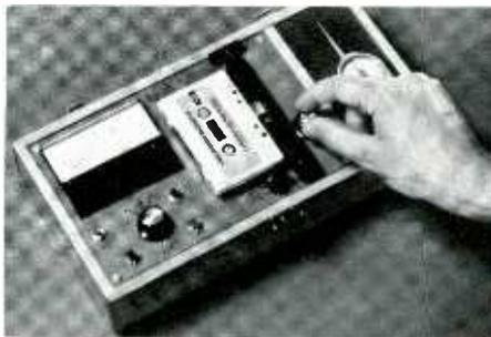
The instrument measures the winding torque in cassettes under varied conditions, and also determines the amount of force exerted on heads by individual pressure pads. The user places a cassette on the instrument's deck, presses the "start" button, and observes the winding torque indicated by the meter.
