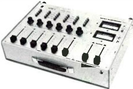
Components used in the Prokit II are from the most prestigious manufacturers including slide pots by Duncan, rotary pots by Allen Bradley, indicator type push button switches by Schadow and input transformers by Jorgen Schou of Denmark. Other features include optional transformer output and optional +48 volt microphone powering.
