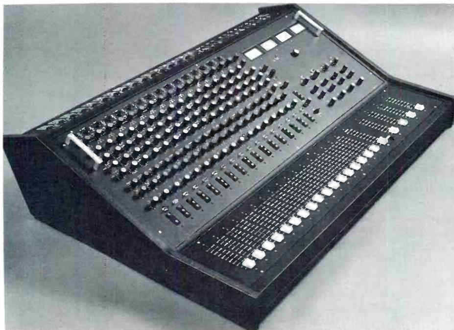
control and "Quasi-parametric" midrange control which permits stepless adjustment of its  $\pm 12$ dB equalization range, as well as continuously variable control over center-frequency and *bandwidth*.
