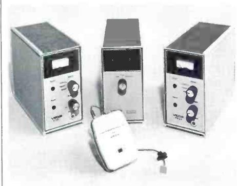
PRO receivers, placed three feet or more apart, both receive the transmissions. Because the two receivers are more than one-half wavelength apart, both will not have signal cancellations at the same instant. Both receivers feed a Model 62 Diversity Combiner that selects the receiver with the best signal strength within microseconds. The switching is immediate and noiseless. The resultant audio, the best of both receivers, is noise free and drop-out free.
