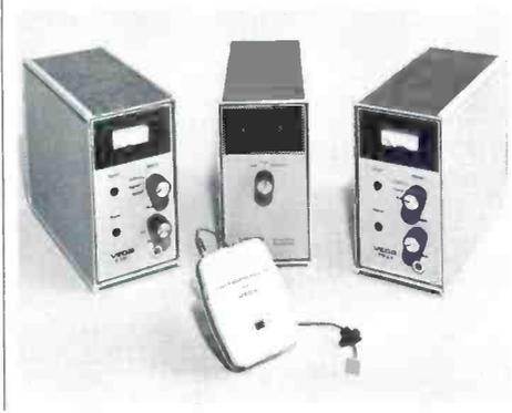
PRO receivers, placed three feet or more apart, both receive the transmissions. Because the two receivers are more than one-half wavelength apart, both will not have signal cancellations at the same instant. Both receivers feed a Model 62 Diversity Combiner that selects the receiver with the best signal strength within microseconds. The switching is immediate and noiseless. The resultant audio, the best of both receivers, is noise free and drop-out free.
