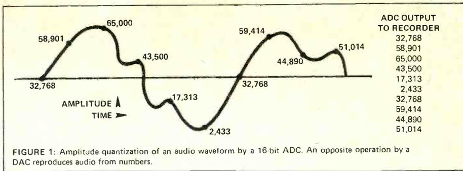
FIGURE 1: Amplitude quantization of an audio waveform by a 16-bit ADC. An opposite operation by a DAC reproduces audio from numbers.
