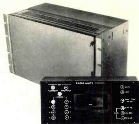
programmer is, in effect, a digital computer including the necessary interface electronics to communicate with the control elements within the console, and also containing sufficient memory capacity to store and retrieve all mixing control data.
