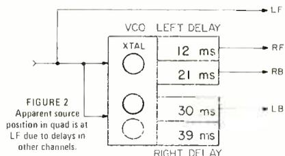
Image placement also involves establishing the source distance. For small differences in distance, as occur when musicians are arrayed front-to-back, we can introduce short delays to the ones that should appear further away. Since sound travels at about 1,100 feet per second, 1 ms corresponds to roughly a foot. This is one of the factors simulated in doubling, as will be discussed later.
