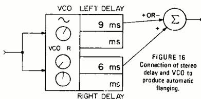
FIGURE 16 Connection of stereo delay and VCO to produce automatic flanging.
