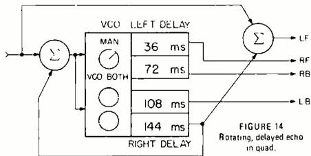
FIGURE 14 Rotating, delayed echo in quad.
