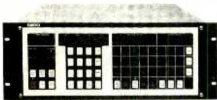
System modes include High Speed Search and Cue, follow the leader or "Chase Mode", Synchronized Play Back, Fast and Slow Re-synchronization and Roll-Back with automatic re-synchronization. Operational efficiency is demonstrated by control simplicity. One button actuates all transports to roll back, start for-
