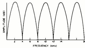
FIGURE 15: Flanging. Characteristic shape for  $t = 0.25$  ms and negative (-) summing on connection of Figure 16. Nulls occur at  $f = 0, 4 \text{ kHz}$  and at  $2, 3, 4 \dots n$  times  $4 \text{ kHz}$ .
