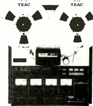
Cawfield said the 40-4 has a combination record/reproduce head, and erase and monitor heads, function and output select buttons, LED overload indicators, accessible calibration controls and a flip-up head cover. The unit has optional four-channel dbx (DX-4), remote control (RC-170) and mike preamp module (MA-4).
