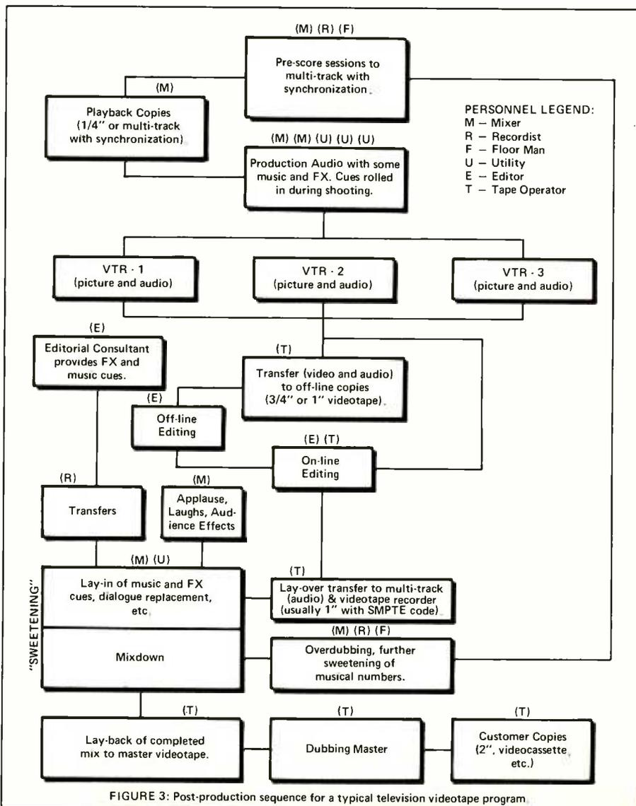
FIGURE 3: Post-production sequence for a typical television videotape program.
