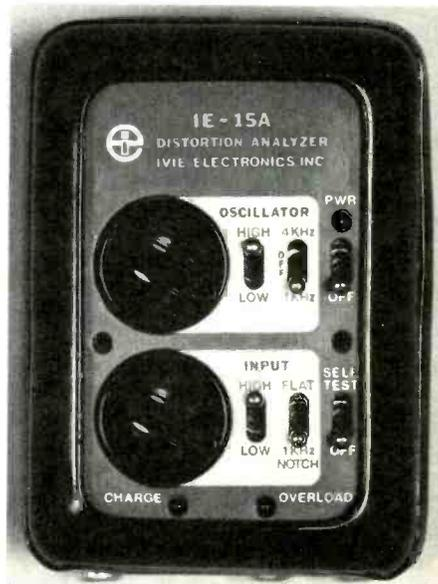
Built into the IE-15A is an ultra-pure sine wave source having selectable frequencies of either 1 kHz or 4 kHz and output voltages adjustable over a 60 dB range. In addition to distortion testing, the oscillators can be used in troubleshooting applications, or in any other task requiring a stable, clean signal source.
