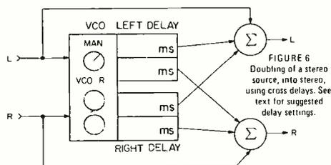
FIGURE 6 Doubling of a stereo source, into stereo, using cross delays. See text for suggested delay settings.
