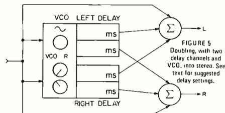
FIGURE 5 Doubling, with two delay channels and VCO, into stereo. See text for suggested delay settings.
