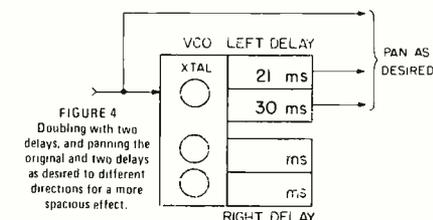
FIGURE 4 Doubling with two delays, and panning the original and two delays as desired to different directions for a more spacious effect.
