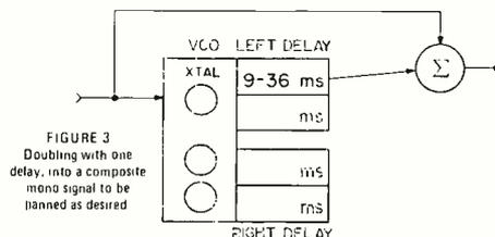
FIGURE 3 Doubling with one delay, into a composite mono signal to be panned as desired
