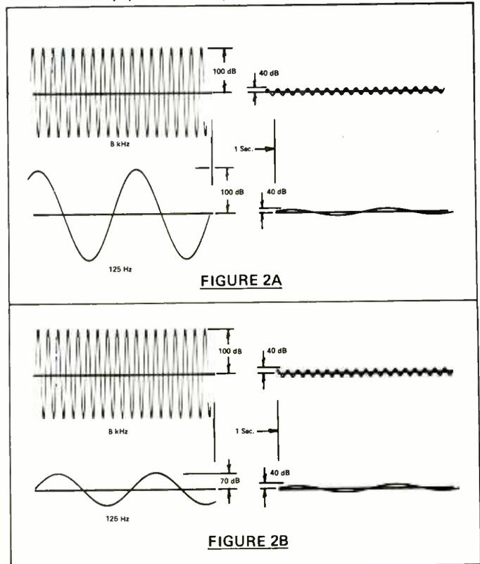
\* $T_{60}$  is defined as the interval in which sound pressure decreases by 60 dB after a steady-state sound has been abruptly shut off.
