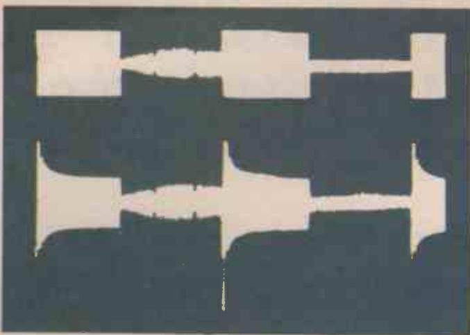
The integrating action of the expander is shown in Figure 2, and is a typical response of this design, to a 25 cycle burst of 1 kHz sine wave. The compression and expansion curves of the compandor are reciprocals of each other and can complement each other without noticeable distortion when connected by a wide band linear transmission system.
