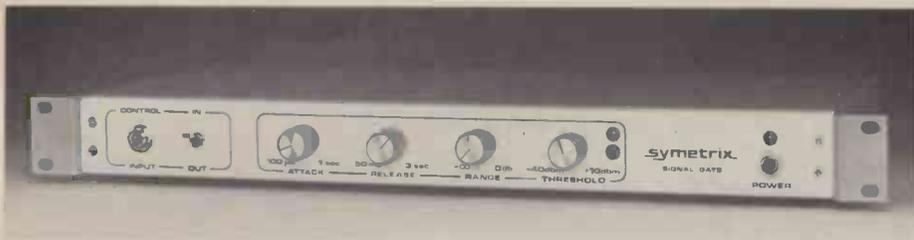
DC control signal. Also mounted on the front panel are two LED's which give a visual indication of the *above or below threshold* status of the program or external control inputs.
