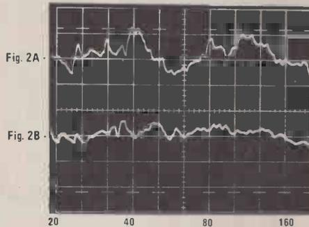
Figure 2A: 1/3rd octave, slow response as in Figure 1A. 20-200 Hz.
