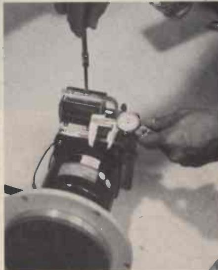
*Ampex brake solenoid travel adjustment*
