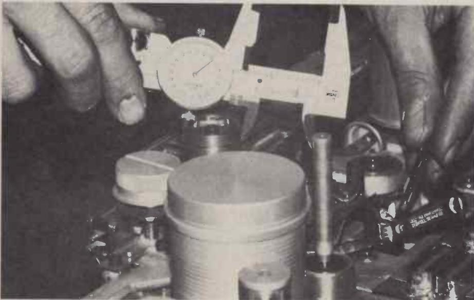
*Studer pinch roller-capstan clearance adjustment.*
