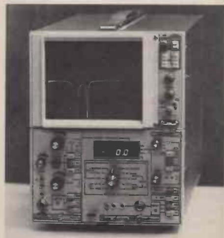
A Tektronix 5111 mainframe houses a series of modular plug-ins including the 301 Generator supplying swept and fixed signals, the 302 Receiver (mono) which digitally displays frequency, level distortion and noise (also controls the storage scope display), and the 306 Stereo Receiver which identifies phase and level differences between two channels.
