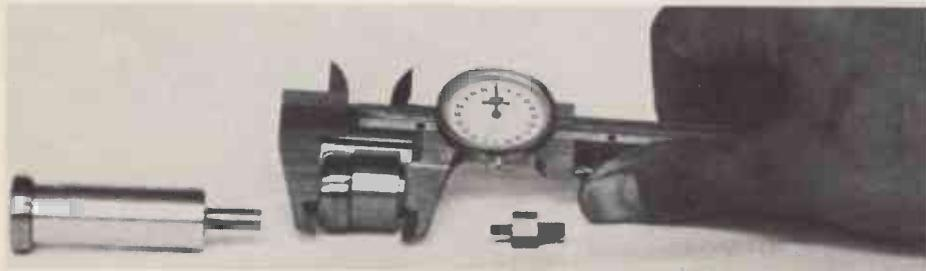
Ampex rotating guide height measurement.
