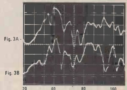
Figure 3A: Long room mode response, 20-200 Hz., sine wave sweep "8".
