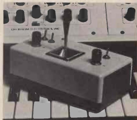
Modification of the sound is realized as the joystick is moved in any direction on a 360 degree horizontal plane. The X axis or left/right of center movement controls pitch bend. The Y axis or forward/backward movement is assigned to filter sweep. Switches are included to allow the player to
