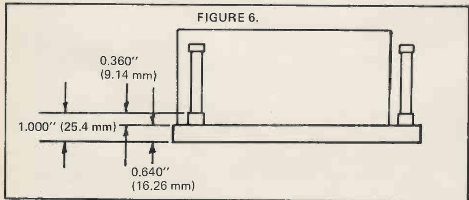
Front elevation view of Ampex head plate and fixed guides.
