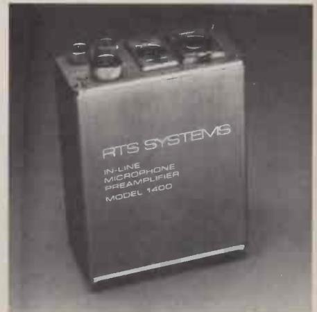
Because the 1400 is battery operated, it avoids a major source of potential hum and ground loops. One pair of 9V batteries form a bipolar supply with an operating life of approximately 100 hours.
