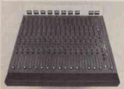
The input modules feature a 4½" conductive plastic slide fader; 6 knob, 3 band parametric equalization; 8/16 track assignment buttons; post echo send; monitor send control; 2 cue sends; solo button which allows stereo panning when engaged; a mic/line switch; and an attenuation switch of -10 or -20 dB.
