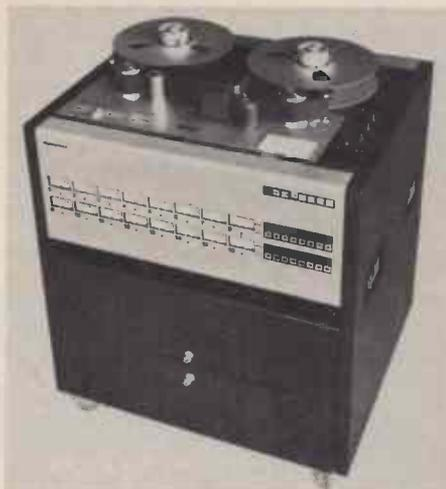
15/30 ips speed configurations and have a tape capacity of 11½", equivalent to 3300 feet of standard tape. Shown is the 16 track version (there is room for up to 32 tracks) with all electronics cards easily accessible in the two file draws beneath. To the right of the top plate are shown capstan speed control and switching for the telcom c4 noise reduction system by TELEFUNKEN which, for up to 24 track configurations, can
