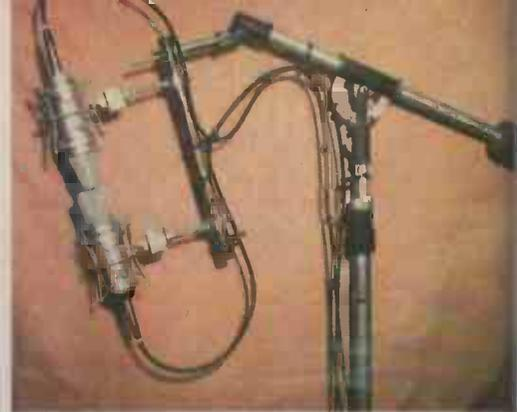
MS (mid-side) microphone assembly showing the extreme close tolerances between the microphone outer cases, as well as the crossarm, counterbalance and adjustable clamp assembly.
