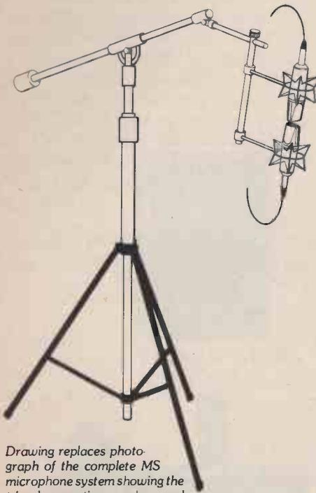
Drawing replaces photograph of the complete MS microphone system showing the tripod supporting members and the adjustable telescopic 1 inch piping.
