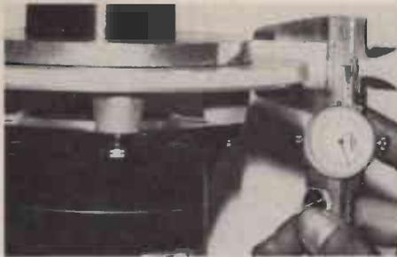
*Ampex reel platform height measurement.*
