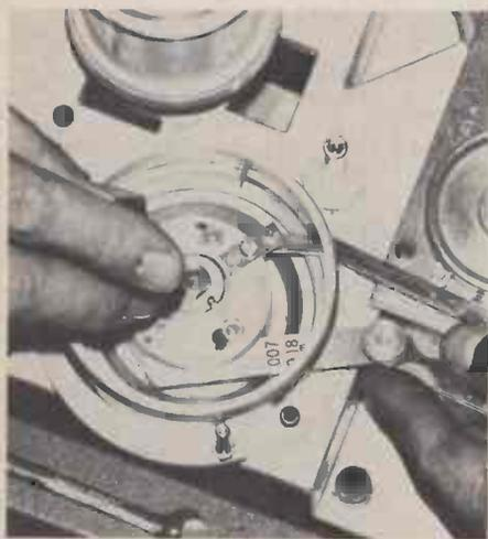
*Studer tension sensor brake armature clearance adjustment.*
