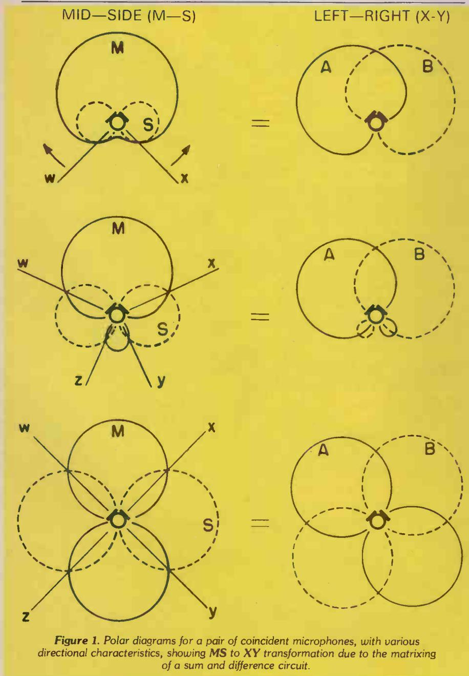
Figure 1. Polar diagrams for a pair of coincident microphones, with various directional characteristics, showing MS to XY transformation due to the matrixing of a sum and difference circuit.
