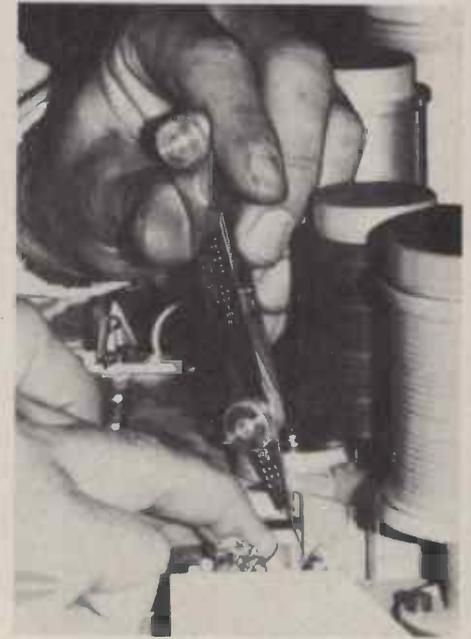
*Studer pinch roller tension arm clearance adjustment.*
