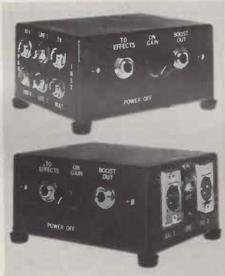
The Universal Hot Box features inputs for instrument level outputs, amplifier speaker level outputs, and line on phone or phono
