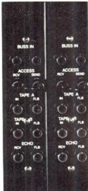
The Model 15 will drive any 16-track recorder and give you a vast array of mixing, monitoring and cueing capabilities. For example, the Cue mixing position can be fed by 48 sources simultaneously (all the inputs plus all 16 tape playback positions plus all eight echo receives).
