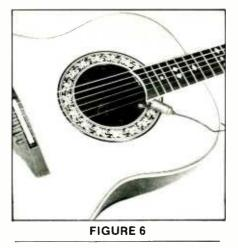
listening panel of eight musicians and audio engineers. In a blind A/B test, the panel compared the tone quality of each close-placed microphone to that of the more distant reference microphone. The majority of the participants considered that a microphone placed next to the sound hole makes the guitar sound bassy, "boomy," "thumpy," and full compared to the timbre picked up at 3 feet; these comments might be expected in view of the spectrum measurement.
