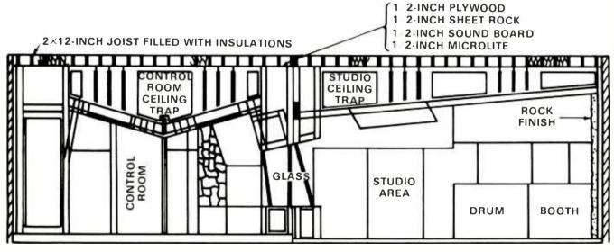
CROSS SECTION OF CONTROL ROOM AND RECORDING AREA
