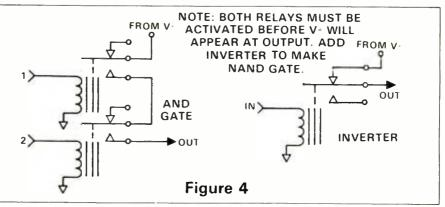
coil is interrupted, and the spring pulls the switch contacts back to the normal state. This activates the coil all over again, and the process will continue to repeat indefinitely. It realize that this is pretty basic stuff although, as I pointed out earlier, so are many logic circuits, or Figures 4, 5 and 6 show relay circuits for AND, OR, and EXCLUSIVE OR gates, whose operation is explained in the next section.
