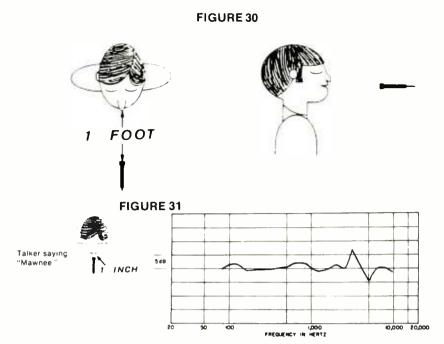
Figure 31: Difference between close-miked spectrum and 1-foot spectrum, for male voice (compare with Figs. 32 & 33 overleaf).
