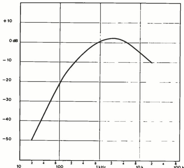
Figure Four: CCIR Weighting Per CCIR 468-2. Unity Gain at 2 kHz Per Dolby ARMS Proposal.
