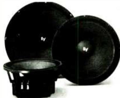
The EVM Pro-Line characteristics are appropriate for both vented (bass reflex) and horn enclosures. Six optimally-vented enclosures have been designed by EV engineers specifically for the new speakers, and span low-frequency limits (3 dB down) from 38 to 83 Hz, and internal volumes from 1.3 to 13.0 cubic feet.
