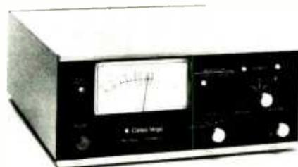
Highest adjacent-channel rejection is achieved with 16 poles of 1F filtering. The preselector is a true four-pole helical-resonator filter (silver-plated). Infinite gain technology is said to ensure the best possible signal-to-noise ratio at low signal levels, and improved processing of multipath RF signals.
