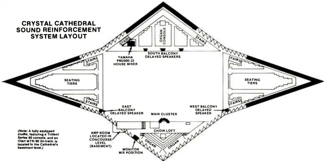
array “put a little too much sound into the side glass panels where there weren’t any seats,” DeLoria recalls. “By reducing that to five cabinets, we got a corresponding reduction in the amount of reverberant field that we excited — and therefore improved intelligibility.”
