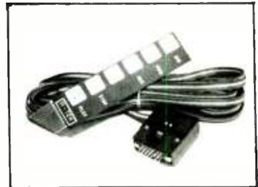
20 foot ribbon cable interface connector allows record, play, fast forward, rewind, stop, and pause functions *without* the need for a bulky remote box.
