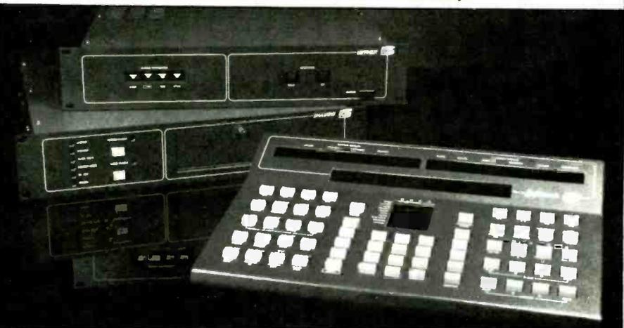
Being software-based, Softouch allows frequently performed multistep routines to be committed to a Softkey memory, and executed repeatedly at the touch of a single key. (The user can define, edit, and store as many as 16 Softkeys at a time during a complex post-production sessions.) Sufficient memory is available to contain all pre- and post-roll, plus "beep-tone" trim, mark in/out, and record in/out data for up to 100 loops.
