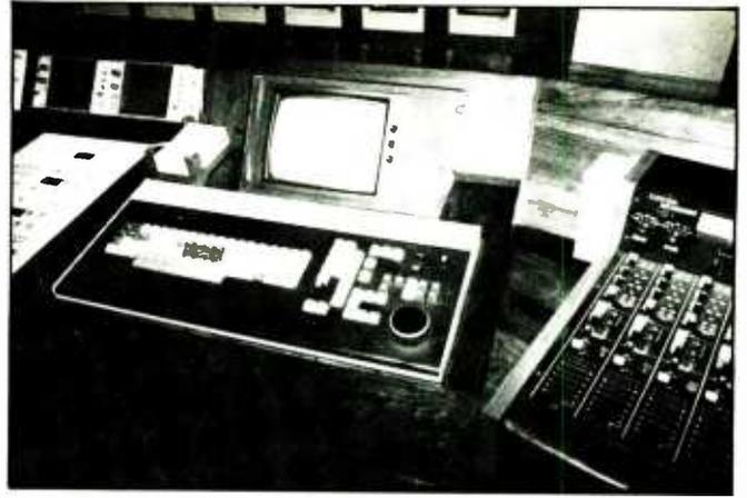
Canyon's Edit 1 houses a Grass Valley 1600-3K video switcher, E-Mem effects memory unit, Harris Epic video editing system, and Quantum QM-8P console. SMPTE timecode locations from the Epic computer control all video transport and switcher commands, plus audio levels via VCA channels.
