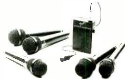
The P-Series of "permanently charged condensers" are said to deliver the wide, flat response and the accurate, neutral sound of studio-quality condenser microphones, plus the ruggedness of a dynamic. The Model P-2 retails for \$99, while the P-1, priced at \$220, features switch-selectable response tailoring, undistorted 150+ dB capability, and internal battery or phantom powering.
