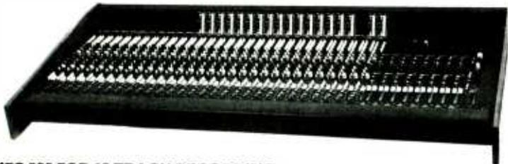
**SERIES 300 FOR 16-TRACK RECORDING:** Series 300 mixers can provide for 16 to 48 Type J or TYPE B input modules (more elaborate equalizers) and frames can be ordered filled or partly filled if desired to be filled later. Dual modular slider track masters have send and pan to monitor, mixer/playback switch, solo to monitor, and effects returns for each track. Type NA stereo control-room monitor module also has outputs for phones and for studio, and talkback/slate.
