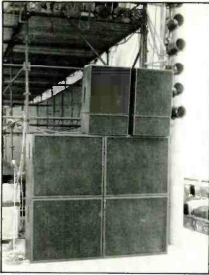
Figure 17: Clair sidefill stacks: 16, 15-inch cones per side, with Community Light & Sound's M-4 diaphragms on the mids, and JBL 2441s on top.
