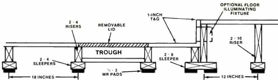
**CONTROL ROOM RAISED PLATFORM AND CABLE TROUGH DETAIL**
