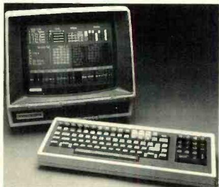
A commercial-grade 16-bit microcomputer and software to form the nucleus of a complete system, which will interface to mixing-console automation, programmable equalization, digital reverberation systems, MIDI, track select, the integration of production paperwork, and a Local Area Network (LAN) to tie together multiple control-room installations and the front office.
