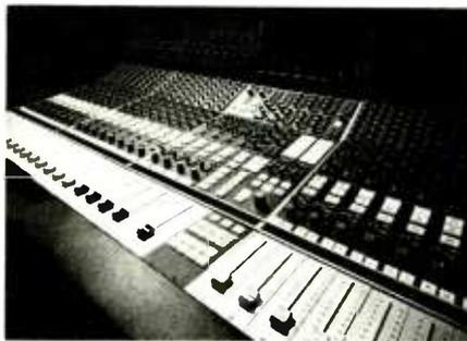
Mainframes for the new system will accept from eight to 56 mono or stereo inputs. Special panning and width enhancement circuitry is provided to simplify the matching of stereo perspective with video. Up to six stereo or 12 mono auxiliary sends may be provided, along with as many as eight stereo IFB/Cue select matrices. (These features are said to speed and simplify the creation of the
