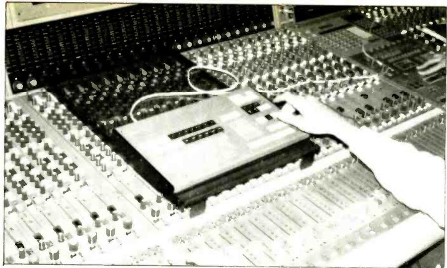
Close up detail of NECAM 96 control panel and keyboard.
