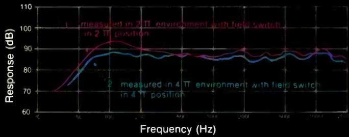
Monitor response will always vary from a 2 pi steradian environment (wall or soffit mounting) to a 4 pi steradian environment (free field or console mounting). The Fostex RM-Series Point Source Monitors provide a front panel Field Switch to provide the same response in both environments.
