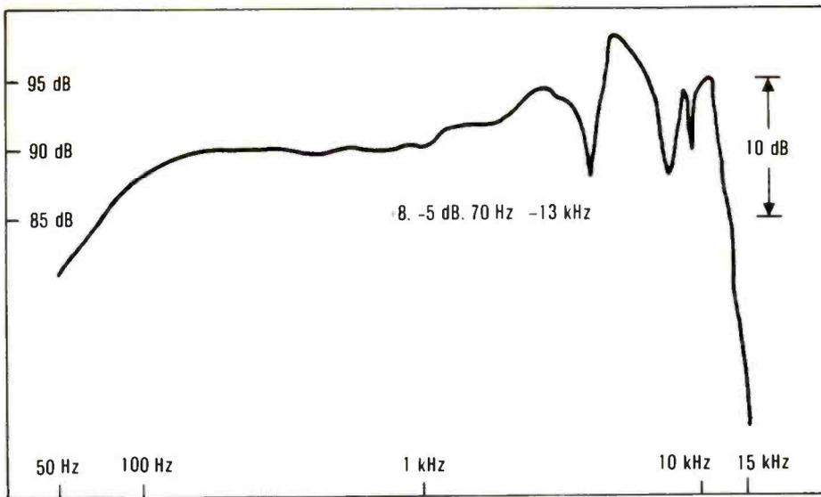
Figure 3: Left earphone response of selected pair of AKG K-141 stereo headphones.
