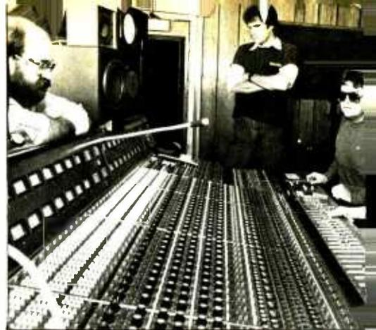
Interior of Ronnie Milsap's Groundstar Studios, equipped with a Neve Model 8128 with NECAM 96 console automation, and two Studer A800 multitracks.
