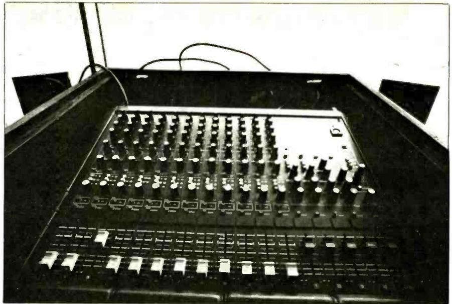
Figure 6: Sound mixing duties at the East L.A. College were handled by a RAMSA WR-8112 console located in a control room that overlooked the playing field.
