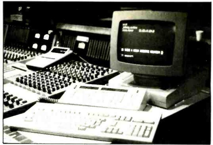
A typical display screen menu (left), plus Conway's keyboard control surface and video display unit. The keyboard (shown in greater detail below) enables labels and annotations to be added to the mix data, and provides enhanced system control.
