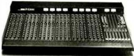
One of the MC Series' unique features is said to be its Input Channel Cue Priority. When an input channel cue switch is pressed, the previous master cue is cancelled. During normal operation, the engineer normally will monitor one of the eight master outputs. If, for example, a feedback problem arises, one or more input channel cue switches can be selected, and the console automatically replaces what was previously being monitored with the new channel's program.
