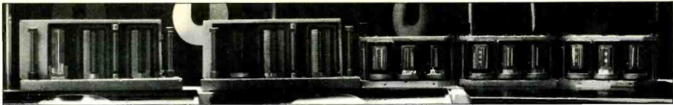
**Tape and Track Formats (L-to-R): 24- and 16-track/two-inch tape, six-, four- and three-track 35mm mag film**
