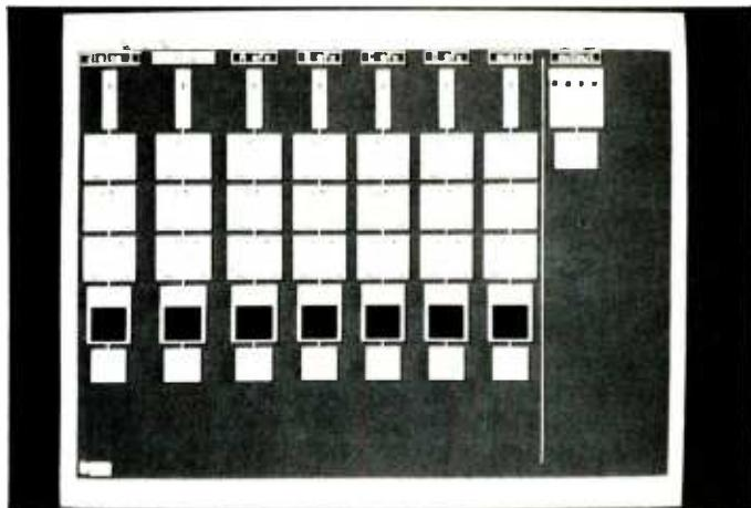
SoundDroid's Electronic Cue Sheet screen (left) indicates audio modulations, start/stop points, and slate information for three tracks simultaneously. Panning, EQ, and reverberation are handled by the Meter Screen (right), and are controlled by eight assignable knobs.
