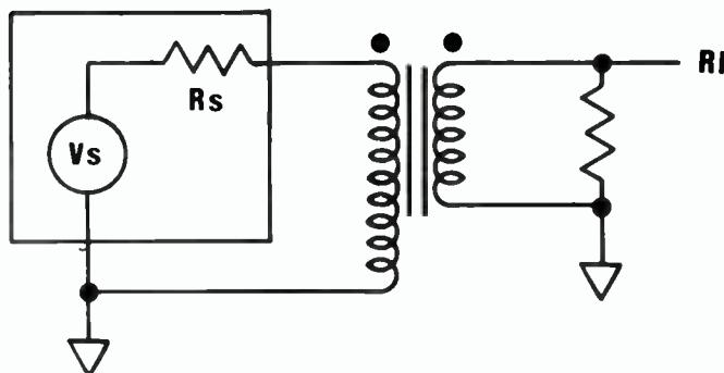
Figure 2: Unbalanced Transformer-Coupled Interface.
