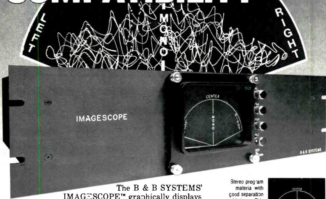
The B & B SYSTEMS' IMAGESCOPE™ graphically displays the complex stereo audio signal, showing you the dispersion of energy as it will sound in the typical listening environment. It gives you an instant indication of L+R phase errors which lead to "flat" and "mushy" mono playback and transmissions. IMAGESCOPE™ is used to position, precisely, any track or tracks within the stereo image. Stereo phase errors are now easily avoided.
