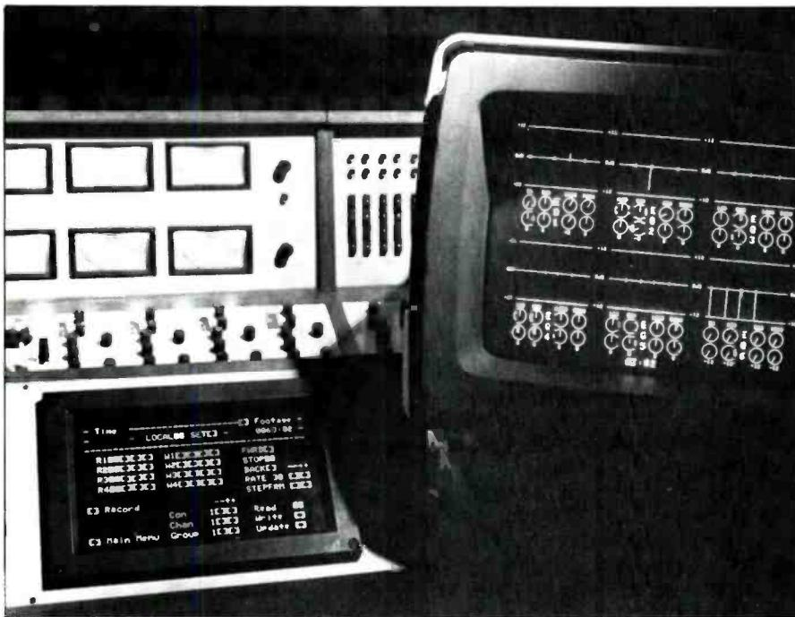
Quad Eight Compumix IV touch-sensitive plasma input/output panel for film re-recording (left), and high-res CRT graphics display of automated parametric EQ.
