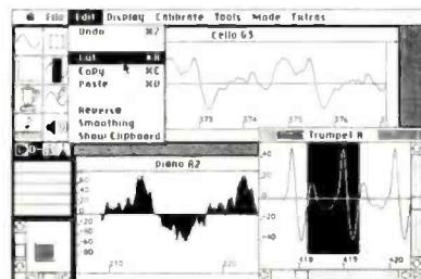
Redraw any part of the waveform using Sound Designer's pencil. Remove clicks or other extraneous noises from sounds by simply drawing them out of the waveform.
