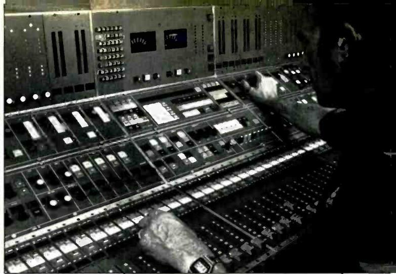
The Neve DSP features central assignment panels (above), multifunction "soft keys" for functional control, and servo-driven faders (right). Shown above right is the 64-channel DSP console delivered to the BBC, England, for installation in a remote truck.
