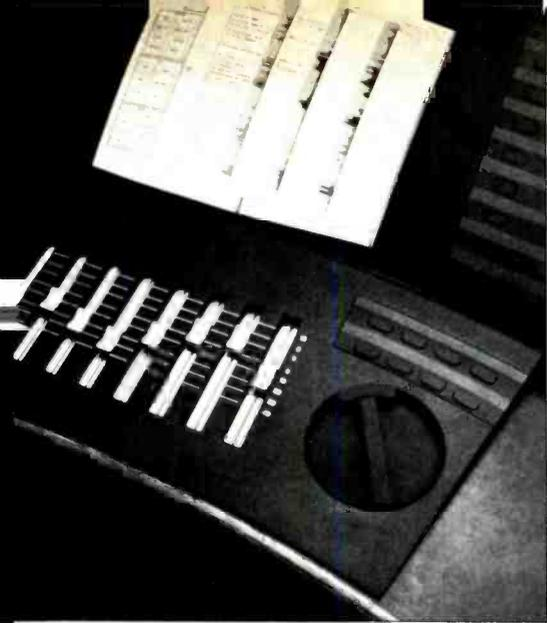
SoundDroid mixing console, featuring GML/Penny & Giles moving faders.
