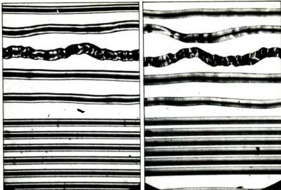
Photomicrograph of mother produced from lacquer master (left) and from DMM copper master (right), showing improved transient response resulting from the "feather-edged," non-heated Direct Metal Mastering cutting stylus.
