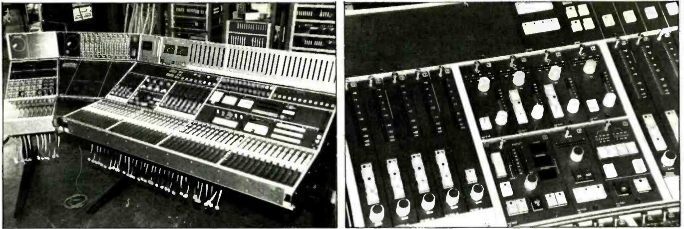
The Audio & Design/Calrec 88-channel digitally-controlled analog console scheduled for delivery to Thames Television, London, England, by late-1985. The central control panel shown in close-up *right* features two assignable sections for EQ, pan, filters, and aux sends, plus assignment functions.
