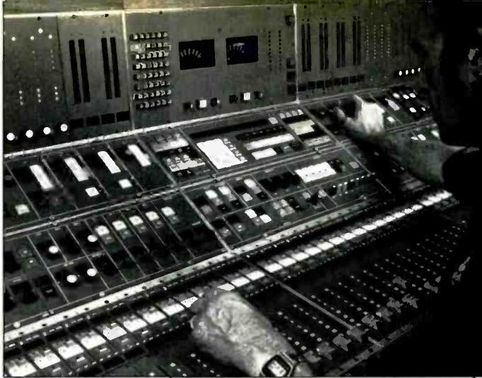
The Neve DSP features central assignment panels (above), multifunction "soft keys" for functional control, and servo-driven faders (right). Shown above right is the 64-channel DSP console delivered to the BBC, England, for installation in a remote truck.
