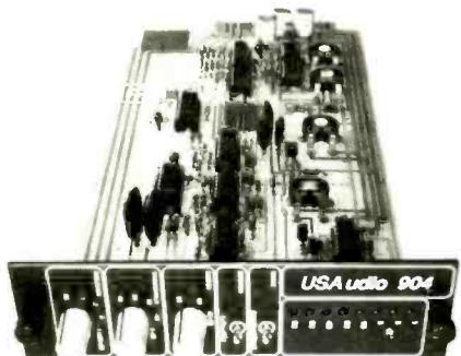
The unit offers two expansion modes, and features an expanded eight-segment LED gain-reduction meter.
