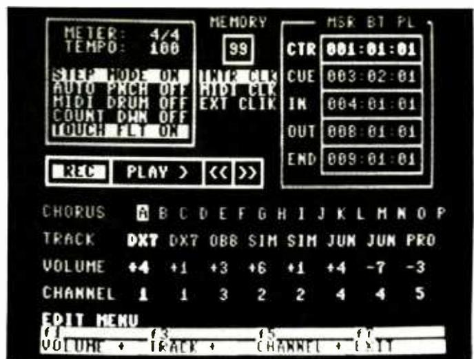
Screen displays for Syntech Corp.'s Digital Studio II software. Shown left is an eight-track song setup menu, while right is a menu for controlling the master "multitrack" controls, MIDI assignments, mode functions, and sequencer data.
