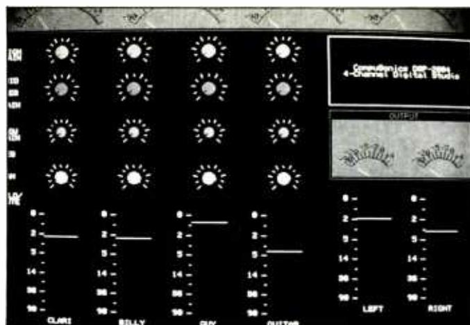
Schematic (left) of the "virtual console" design of the CompuSonics DSP-2000 Series mixers/recorders. At right is the CompuSonics console screen, with all of the "knobs" and "faders" controlled by trackballs. These screen graphics are in full color.
