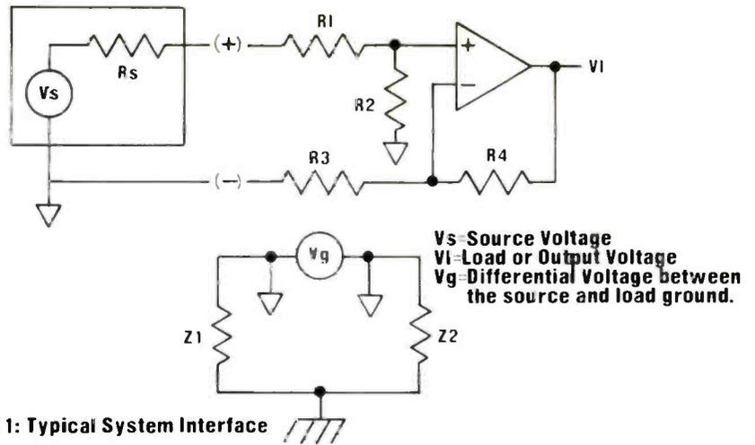
Figure 1: Typical System Interface
