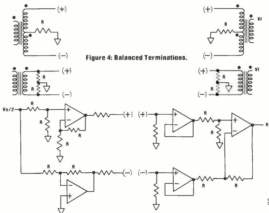
**Figure 4: Balanced Terminations.**
