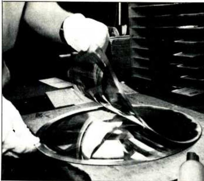
During preparation of the DMM copper blank, a stainless steel substrate receives a 4-mill coating of pure copper (left). At the matrix-preparation facility, a nickel stamper is "grown" directly by electrolysis from the copper mother.
