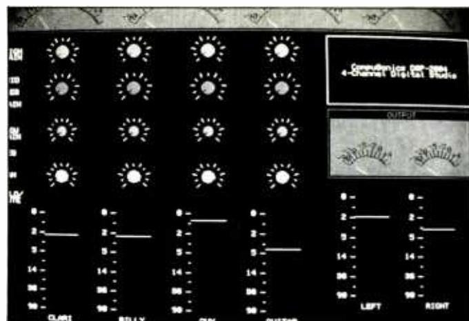
Schematic (left) of the "virtual console" design of the CompuSonics DSP-2000 Series mixers/recorders. At right is the CompuSonics console screen, with all of the "knobs" and "faders" controlled by trackballs. These screen graphics are in full color.
