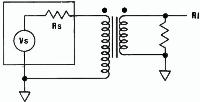
Figure 2: Unbalanced Transformer-Coupled Interface.
