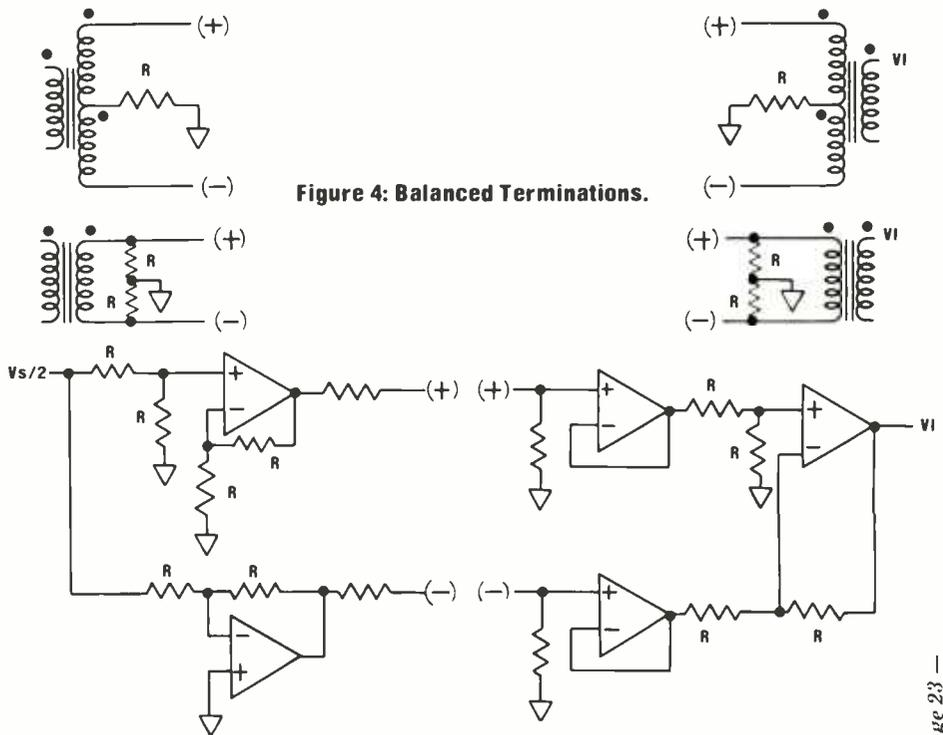
Figure 4: Balanced Terminations.
