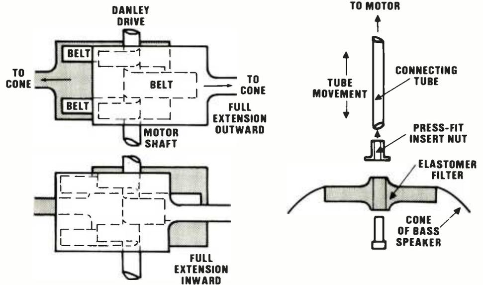
Figure 1: A rotary-to-linear converter drives the speaker cones in the Intersonics SDL units. An electric motor's power is transferred to the cone with a "drive shaft."
