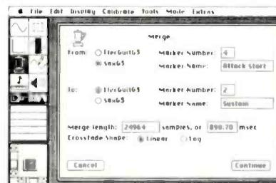
The essential process of looping sampled sounds is greatly simplified by Sound Designer. No more random (and time consuming) searches for loop points—you can see the waveform and quickly assign the loop in the proper location.
