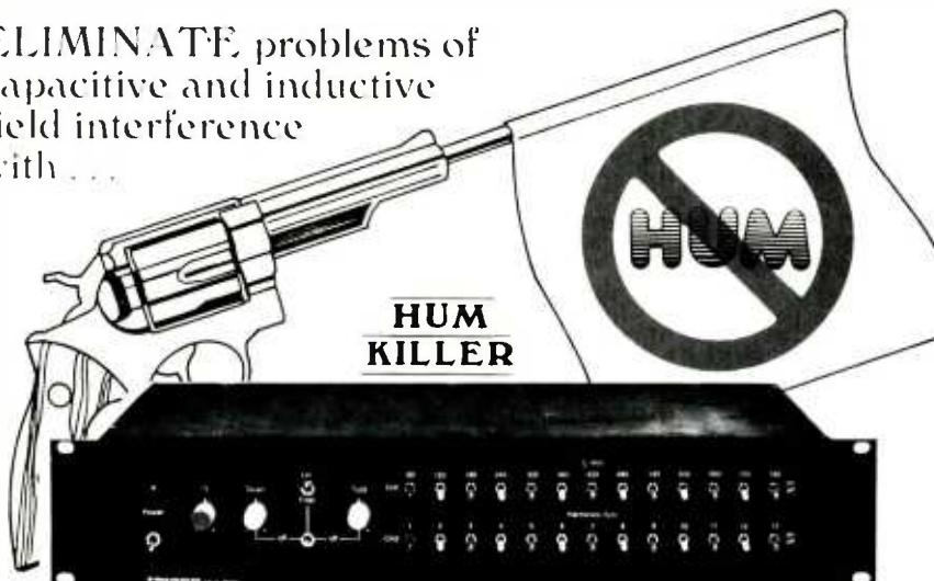
The HUM-KILLER influences both the even and odd harmonics up to the 13th harmonic with the use of thirteen extremely narrow-band filters affecting the low-frequency signal ranges. These filters, including the filter for the fundamental wave, have a bandwidth of only 6%. (For the 50 Hz model the bandwidth is 3 Hz.) In operation, filters can be added one by one, thus making it possible to isolate and exactly detect, and eliminate the disturbing hum or
