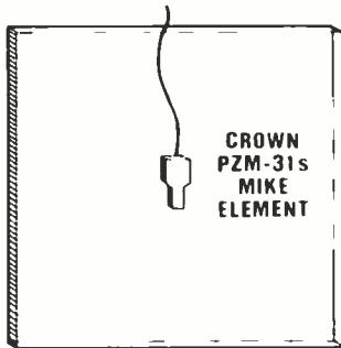
ABOVE: CLOSE-UP DETAIL OF STEREO ARRAY USED DURING BUDDY RICH AUDIO/VIDEO SHOOT. THE ARRAY MEASURES 12 BY FOUR FEET, AND IS MADE UP FROM 4-BY 4-FOOT PLEXIGLASS SHEETS.
