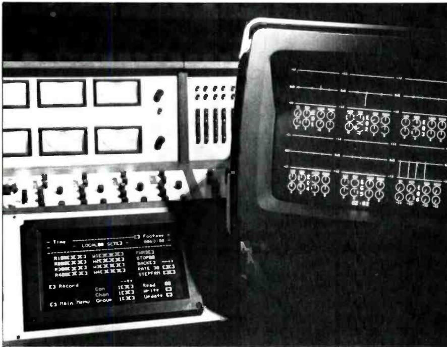
Quad Eight Compumix IV touch-sensitive plasma input/output panel for film recording (left), and high-res CRT graphics display of automated parametric EQ.
