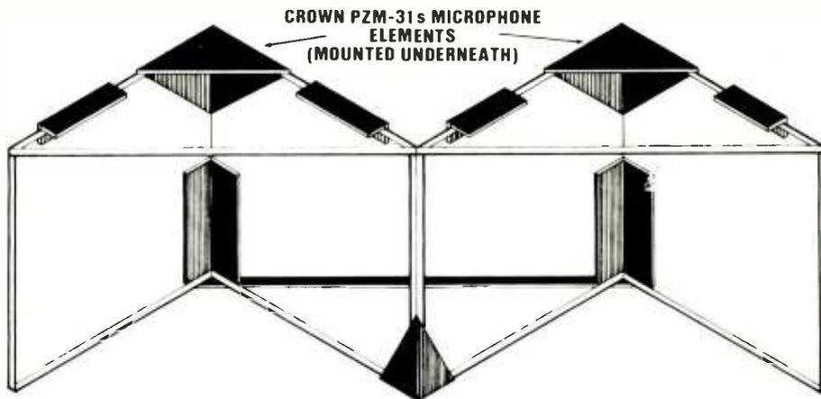
**ABOVE: CLOSE-UP DETAIL OF STEREO ARRAY USED DURING BUDDY RICH AUDIO/VIDEO SHOOT. THE ARRAY MEASURES 12 BY FOUR FEET, AND IS MADE UP FROM 4- BY 4-FOOT PLEXIGLASS SHEETS.**
