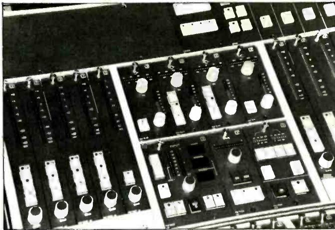
The Audio & Design/Calrec 88-channel digitally-controlled analog console scheduled for delivery to Thames Television, London, England, by late-1985. The central control panel shown in close-up right features two assignable sections for EQ, pan, filters, and aux sends, plus assignment functions.
