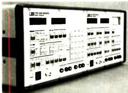
Test results are achieved in less than 60 seconds, and may be graphed on a standard printer or plotter. If desired, the 3000 Series functions may also be controlled via RS-232C or GPIB (IEEE-488) communications ports.
