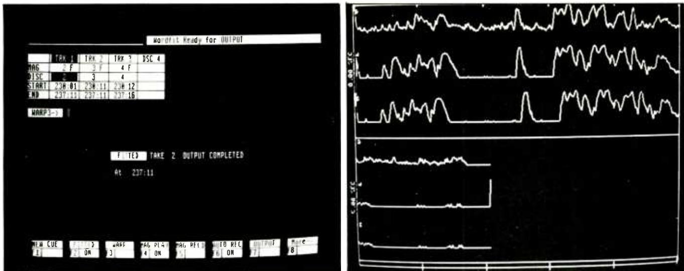
**Wordfit ADR system screens.** Left is the operating menu; at right are traces of the guide track (top), fitted track (center), and unfitted track (lower). One screen width is equal to five seconds; the next two seconds of all three tracks are on the bottom half of the screen.
