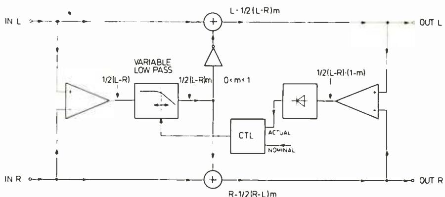
BLOCK DIAGRAM OF NEUMANN VAB-84 VERTICAL AMPLITUDE LIMITER
