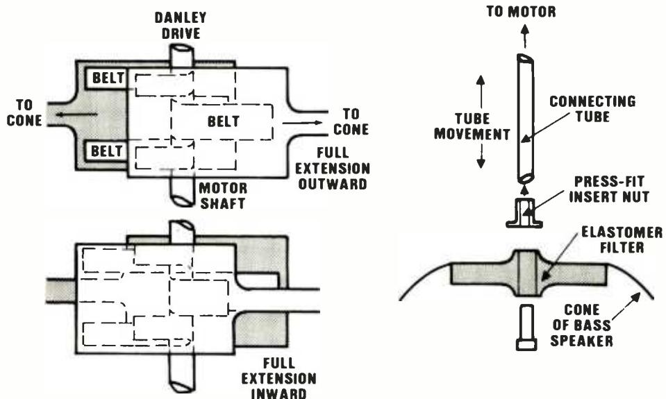
Figure 1: A rotary-to-linear converter drives the speaker cones in the Intersonics SDL units. An electric motor's power is transferred to the cone with a "drive shaft."
