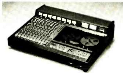
SMPTE/EBU synchronizers and controllers are plug-compatible with an accessory jack fitted to the Studio 8, making it an ideal system to introduce high-quality eight-track audio to the sync-video market, at a very low cost. Also, composers working in
