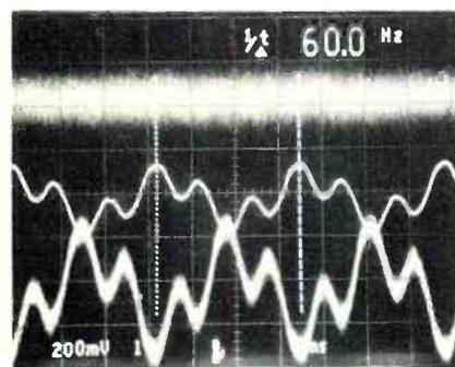
**Figure 9.** The top trace is the residual program noise output and measures  $-88.5dBu$ . With  $1.2mA$  of ground current flowing (center trace), the output noise floor (bottom trace) rises to  $-74.5dBu$ , an increase of  $14dB$ .
