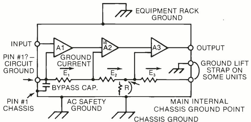
Figure 4. A shield connected to the circuit ground, shield or ground currents (at one end only) will cause the voltage drops  $e_1$ ,  $e_2$  and  $e_3$ , which are amplified by  $A_2$  and  $A_3$ . Sometimes a small resistance,  $R$ , connects the chassis and the circuit ground, reducing these voltages.
