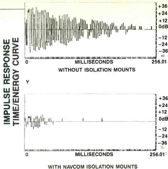
Figure 2. Relative energy/time plots for vibration leakage to the floor with and without isolation.
