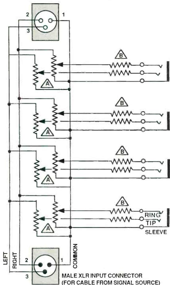
**A** HEAVY DUTY VERSION: USE TWO 100 OHM, 12 WATT POTS PER OUTPUT JACK (L, R); Ohmite 0112 or equivalent.
