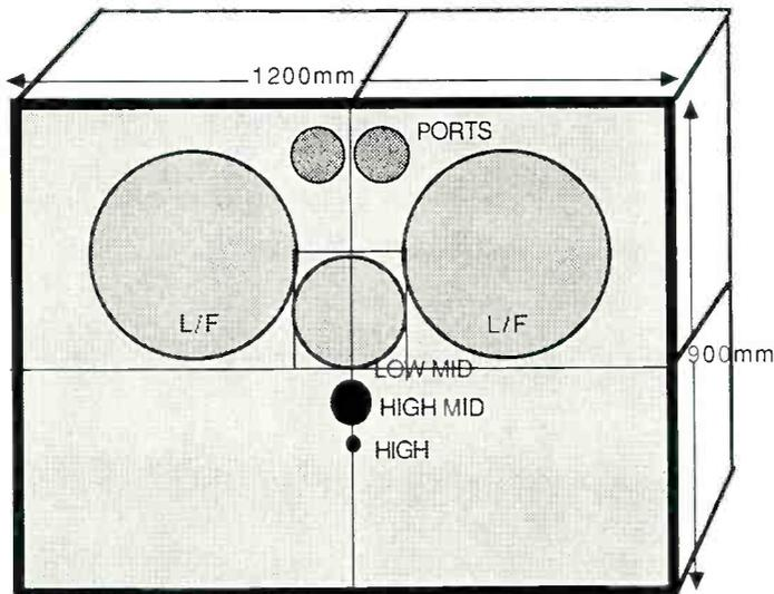
System layout of the M4(5). This view represents the front panel with all units flush-mounted.
