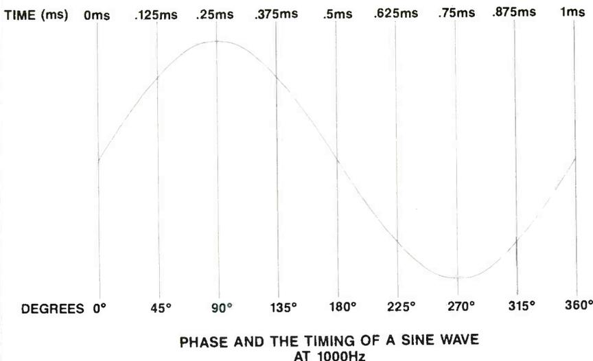
Figure 1. Phase and the timing of a sine wave AT 1,000Hz.
