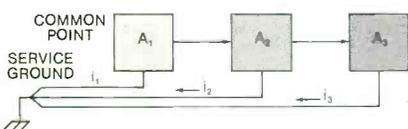
**Figure 8.** In a star or unipoint ground, with isolated safety ground, the ground currents do not add up because all the grounds are referenced to one point. To function properly, the point cannot be 50 feet long, but should be a proper ground bus in the power-service panel.
