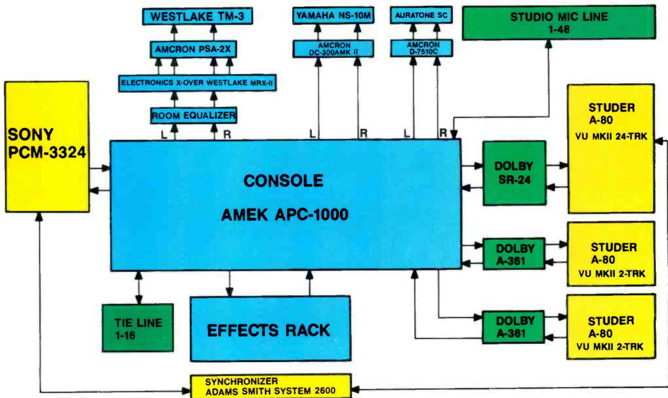
Figure 2. Equipment layout for Studio Jive.
