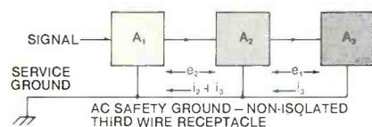
**Figure 7.** Serial ground implementation. Equipment-leakage currents flowing in the safety ground create small potential differences among the equipment. Amplifier A multiplies the ground current by its gain.
