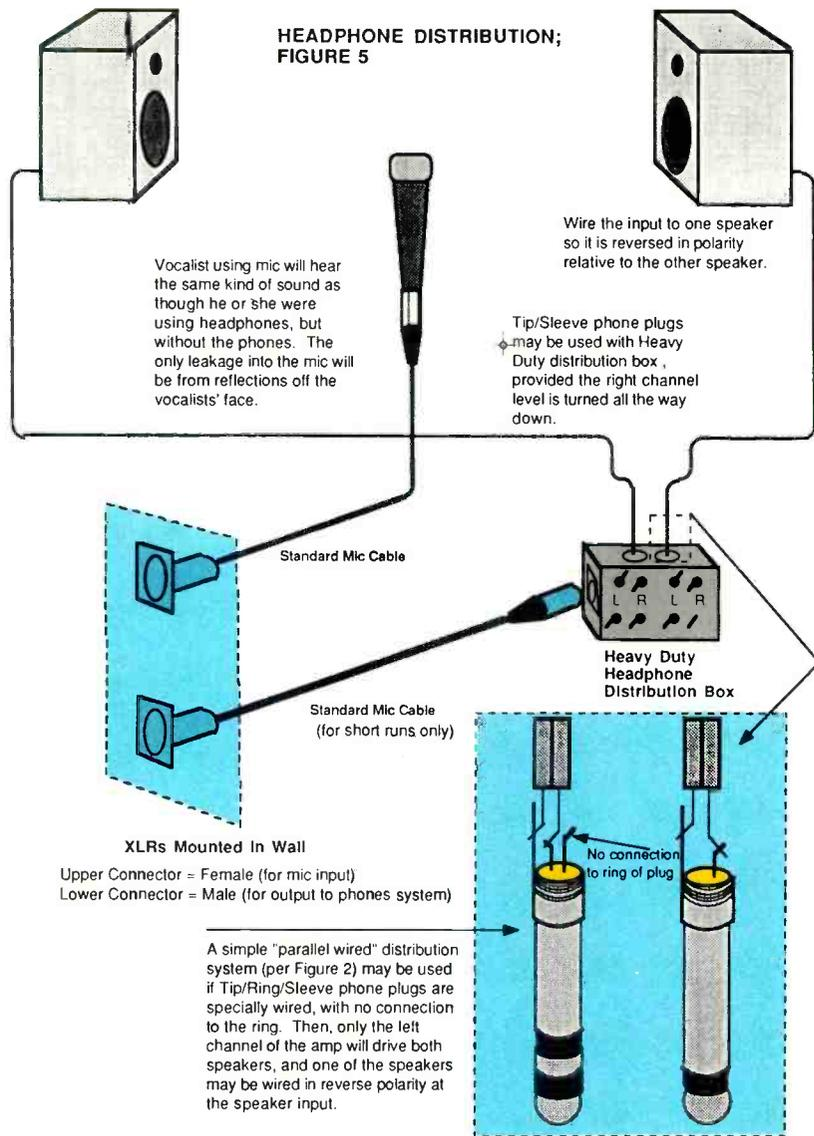
**Figure 5.** Pictorial of headphone distribution system used to drive reverse-polarity speakers to eliminate cue phones.
