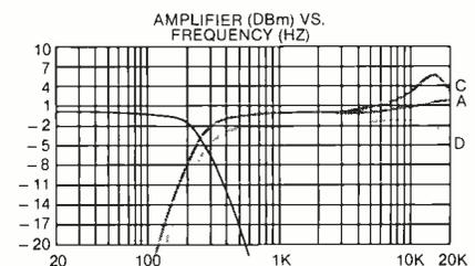
Figure 6. Swept frequency-response curves showing the effects of cable loading on an electronic crossover. The frequency response in curve C shows that ringing outside the audio band does affect what happens inside the audio band.
