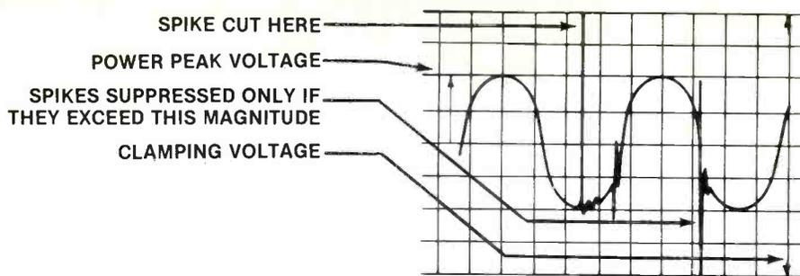
**Figure 2.** Spike clippers suppress only voltage spikes that exceed the clamping voltage, which is customarily set at approximately 200Vac for a nominal 120Vac power line.
