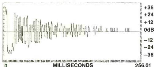
NON SERVO- SERVO TURNED OFF, AND NO ELECTRONIC CROSSOVER. (UNIT PERFORMS SIMILAR TO A CONVENTIONAL NON-SERVO SUBWOOFER).
