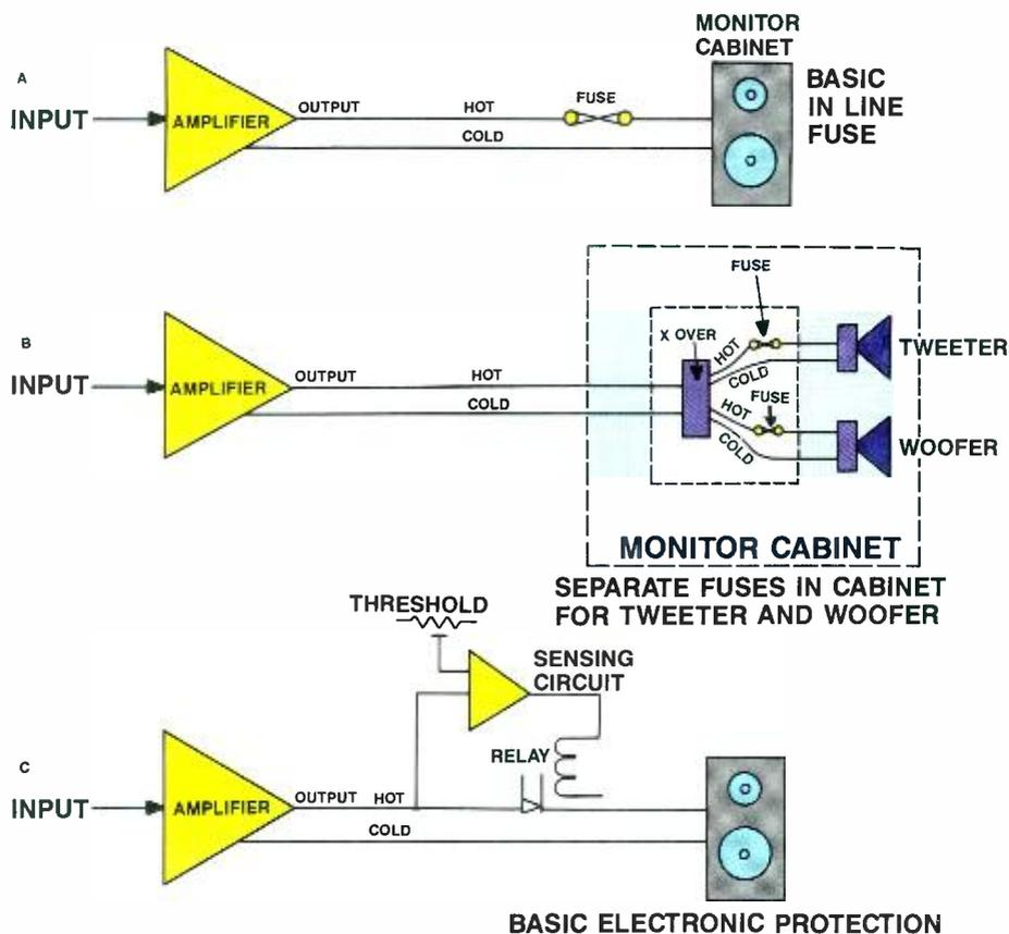
**Figure 2.** A: Example of in-line fuse between the amplifier and the monitor. B: Example of fuses fit inside the cabinet. C: Example of electronic protection.
