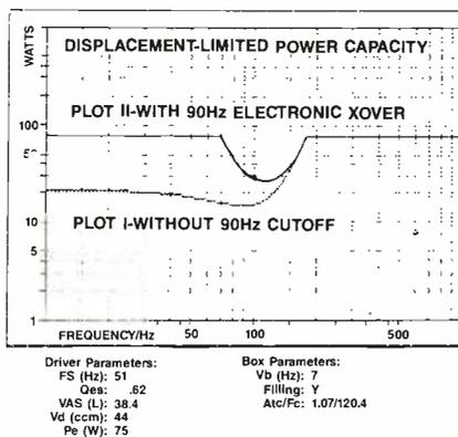
Figure 1. Yamaha NS-10M power and handling model with and without high-pass electronic crossover.
