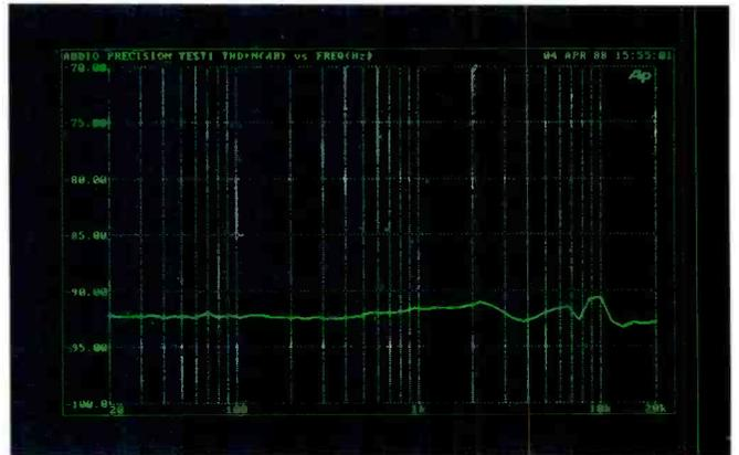
Using an Audio Precision system, a sine wave is processed through sample and hold, A to D, ZAD2716 A/D converter, and Apogee AP filter. Graph shows combined total harmonic distortion and noise vs. frequency.
