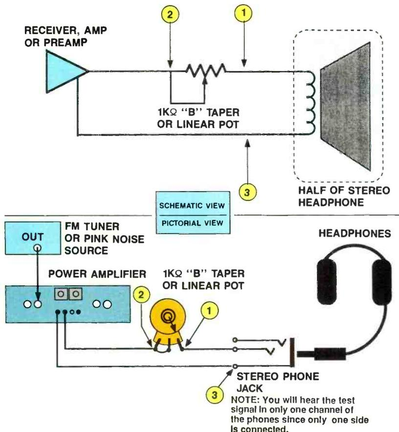
Figure 1. Test setup for measuring headphone impedance.
