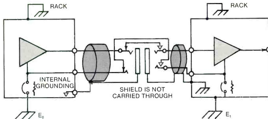
**Figure 11.** Unbalanced I/O through a patchbay. How the grounding is handled inside the units determines the overall result. The larger the difference between  $E_0$  and  $E_1$ , the worse the problem. To ensure success, both units should be plugged into the same duplex outlet, operating from the same phase. Often the unbalanced I/O is a normalized send/receive loop on a console remote to a patchbay.
