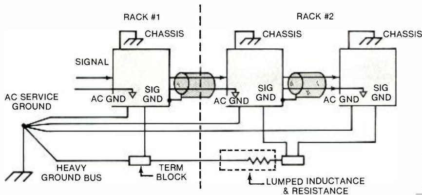
**Figure 10.** Concept of a technical ground implemented with a low-impedance ground bus. The theory holds only if the technical ground's actual impedance is considerably below the rest of the signal return paths.
