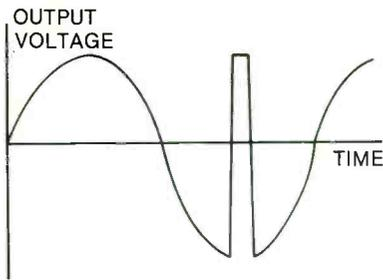
**Figure 2.** When an amp that uses a Bi-FET op-amp at the input receives too much common-mode voltage, the output reverses itself and swings in the opposite direction.
