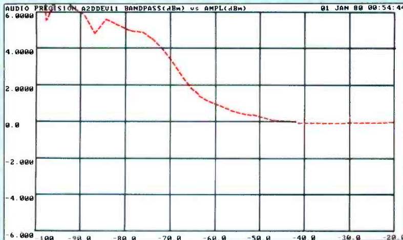
Figure 3. Deviation from linearity, poor channel (channel 11).
