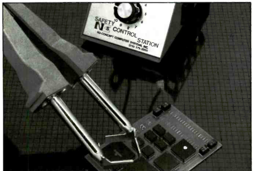
The control station, shown in the background, allows the probe tip temperature to be carefully controlled to prevent damage to the ICs.
