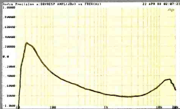
Figure 3A. Frequency response of dbx system, no ATR. (Note expanded scale of \pm 1\text{dB} .)
