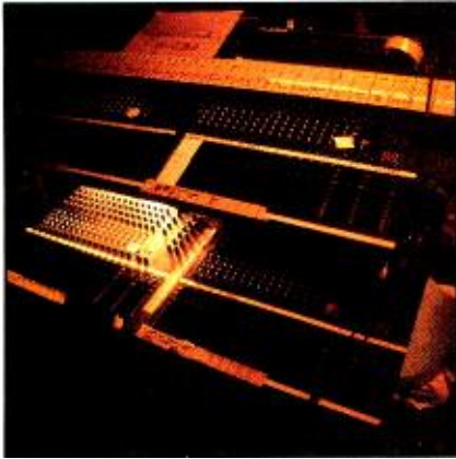
Figure 4. Four Alesis 1622 mixers were held in place by a custom rack. The top two units were on a hinged panel, allowing quick access to the lower pair with little effort on the part of the sound mixer.
