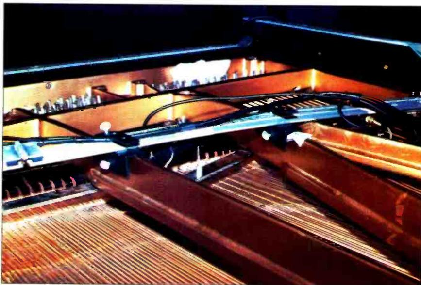
Figure 2. Customized Helpinstill pickups and pre-amps provided a high-quality amplification of Bruce Hornsby's piano without using any microphones.
