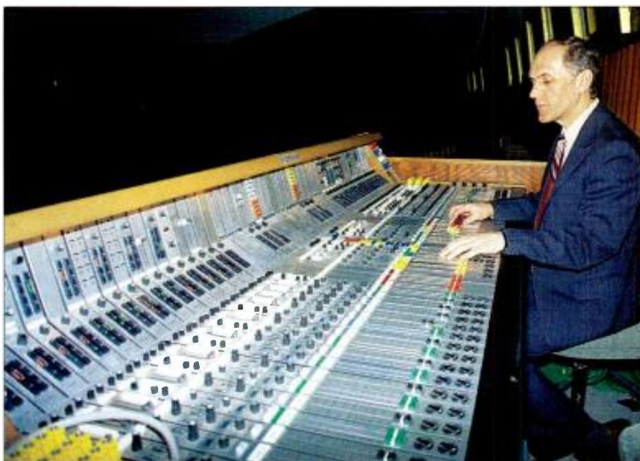
*Installed in 1985, the Kremlin Palace's Siemens mixing console is 27 feet long. Operated by staff tonmeisters, the console has separate sections with different input and output modules to serve lecture, theatrical and orchestral events.*
