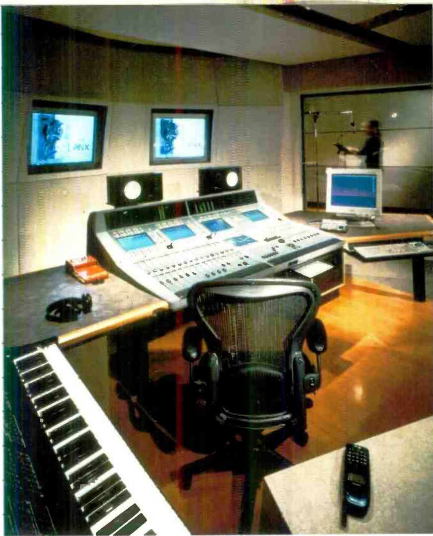
▲ US: Manhattan's Photomag post house has added a second Soundtracs DPC-II digital console in its downtown Photomag@The Anx facility. The recently refitted Studio A will see the new DPC-II working alongside a Fairlight MFX3+ and is 5.1 equipped. Photomag 'Partners in Sound', US. Tel: +1 212 687 9030.
