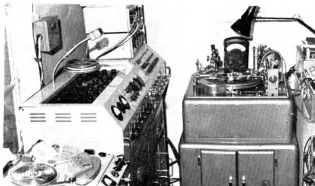
Trusound disc-cutting installation
