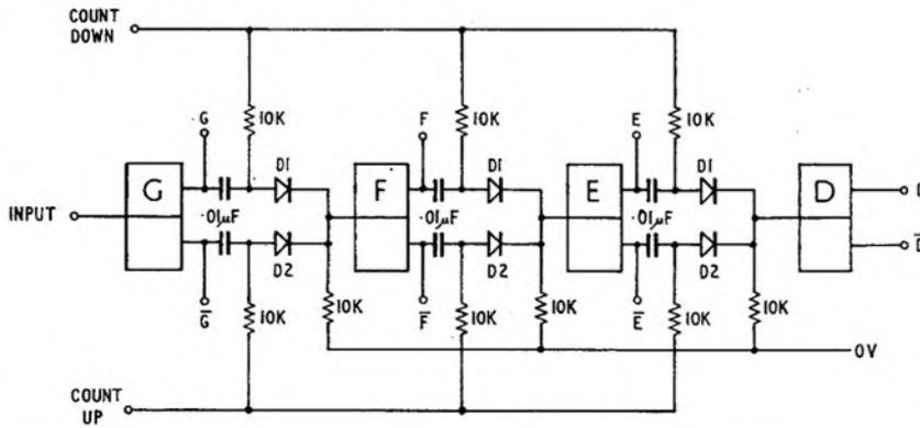
FIG. 10 BINARY TO 1 OF 16 CONVERTER
