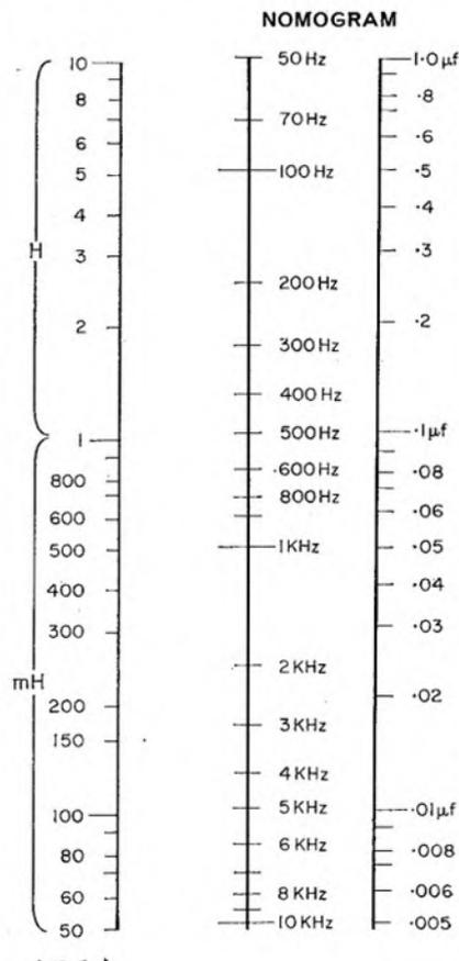
PLACE A STRAIGHT EDGE BETWEEN SELECTED VALUES IN ANY TWO COLUMNS AND READ OFF THE THIRD, UNKNOWN PARAMETER IN THE REMAINING COLUMN. FOR COIL WINDING DETAILS SEE TEXT L.H. COLUMN
