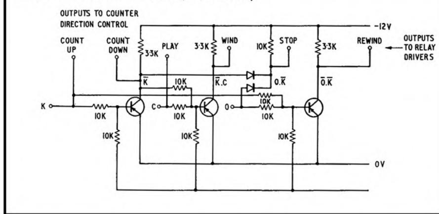
FIG.15 TAPE DECK CONTROL CIRCUIT (WITH DELAYS)
