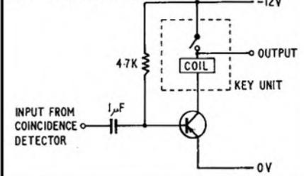
FIG. 12 KEY PRESSED AND COINCIDENCE DETECTORS
