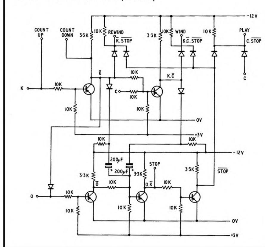
FIG. 16 EXAMPLES OF RELAY LOGIC
