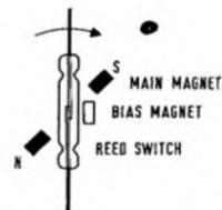
ROTARY SWITCH WITH BIAS MAGNET WILL GIVE ONE PULSE PER FRAME
