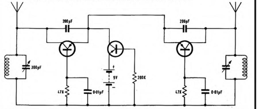
**FIG. 25 BISTABLE MULTIVIBRATOR FREQUENCY DIVIDER, USING DIODE STEERING**
