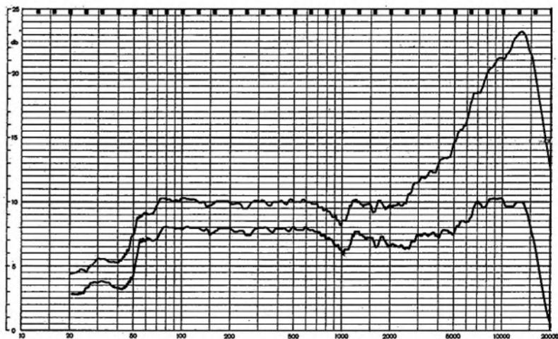
B & K frequency response traces with 0.25  $\mu$ F capacitor at output (lower curve) and without capacitor.
