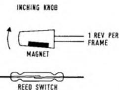
MAGNET GLUED TO INCHING KNOB TO GIVE ONE PULSE PER FRAME
