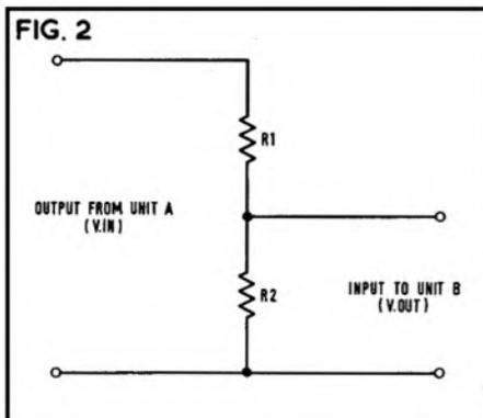
Thus, we have now overcome most of the problems likely to occur with impedance matching. It should be remembered that if an input impedance is stated as 10 K it means that we can safely apply any input load up to this value without degrading performance. If there is sufficient feedback in the circuit it means that the value of the input impedance can well exceed the 10 K value without detriment to the circuit. However it is not advisable to work an amplifier under such conditions.
