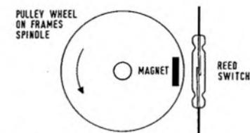
ROTATING MAGNET GLUED TO PULLEY WHEEL TO FORM A CAM SWITCH
