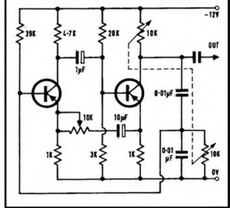
FIG. 12 TWIN-T FEEDBACK OSCILLATOR
