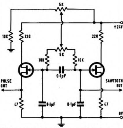
(c) VARIABLE-SPACING PULSE AND DUAL-AMPLITUDE SAWTOOTH OSCILLATOR
