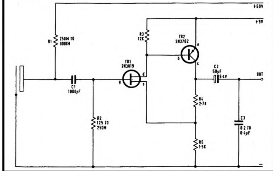
FIG. 1 REVOX G36 CIRCUIT DIAGRAM
