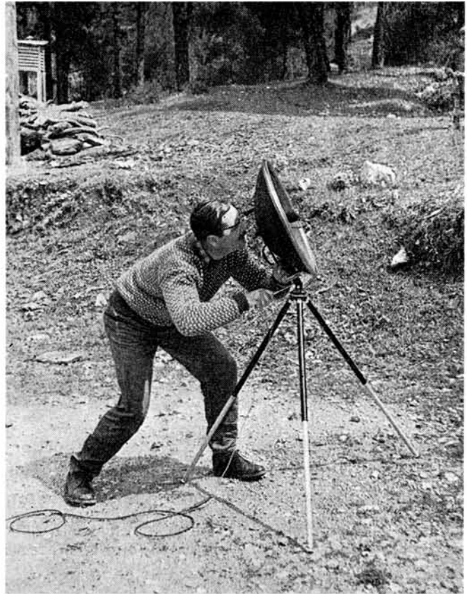
The author is seen sighting the parabola to record bird song on a recent expedition with naturalist/photographer Eric Hosking. The parabola's directional properties are particularly useful for picking up distant sounds.
