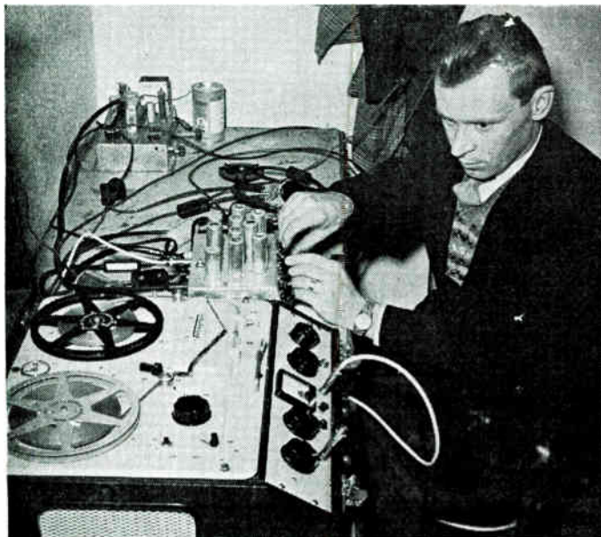
Les Wake is a recording engineer with R.S.C.A. Recordings, Thanet, and something of a genius at producing gadgets and special effects. The electronic mixer, seen here in use with a Ferragraph is all his own work.
