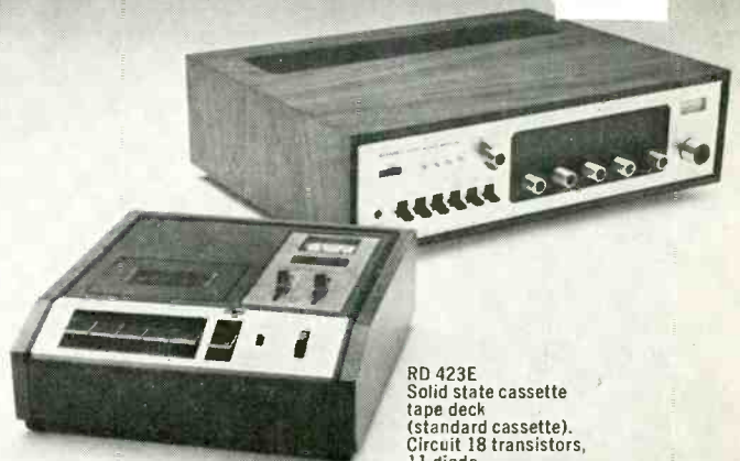
STA 32L Solid state stereo tuner/amplifier. Circuit 42 transistor (including 3 FETs) 1-1c, 28 diode. Type MW/LW/FM multiplex 3 band superheterodyne stereo tuner/amplifier. Tuning range 525-1605kHz, LW 150-370kHz, FM 88-108 MHz. Output 80W (40W + 40W) max. music power £115.00
