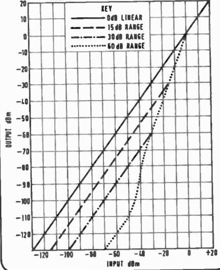
FIG. 2 EFFECT OF THRESHOLD CONTROL ON EXPANSION CHARACTERISTICS
