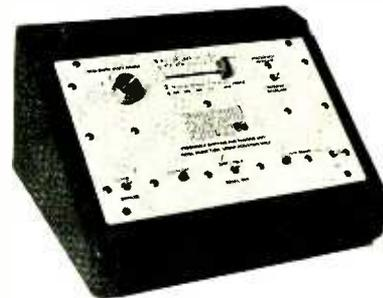
Shifts the audio spectrum upwards or downwards by any amount between 0.1 and 1000 Hertz for weird effects on music or speech. Unlike any other form of signal processing, the shift of all audio frequencies by the same number of Hertz destroys the normal harmonic relationships.
