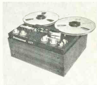
3.77 Based on the A77 chassis and introduced at the request of the recording industry to meet their requirements of 3-speeds, full editing facilities, motion sensing and immediate access to the heads. Designed and rebuilt by ITA.
