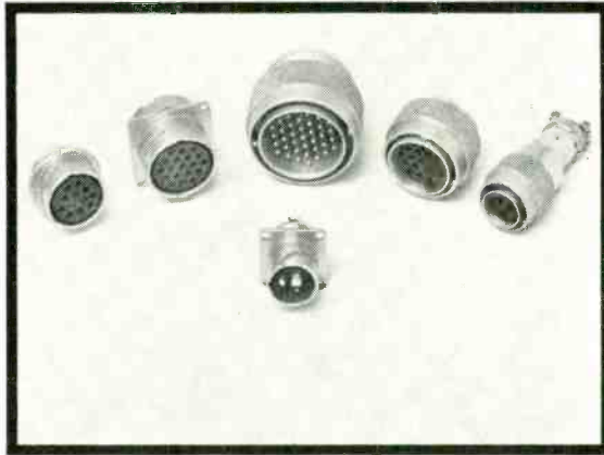
SOURIAU. We stock two ranges – the 8400 circular bayonet-locking type (illustrated) available in 1-37 ways in five shell sizes and the 8291 rectangular series to MIL-C-28748. The 8291 is interchangeable with other types to this specification and features metal shrouds, jack-screw locking, four contact types including co-axial and is available up to 104 ways.
