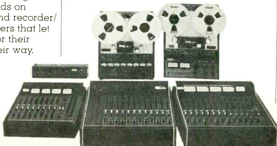
The Model 5-EX shown with four optional 201 input modules. Model 5 shown with optional 204 talk back/slate module.
