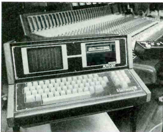
Above: Harrison's Auto Set control unit and microprocessor
