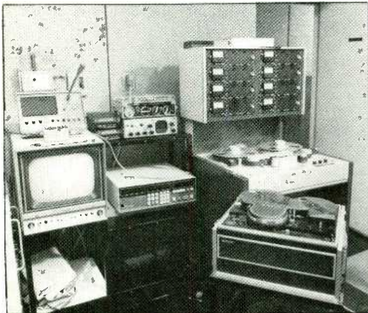
Central Dynamics ED200 being used at Ewart Studios to synchronise Sony Video tape recorder and A80 8-track
