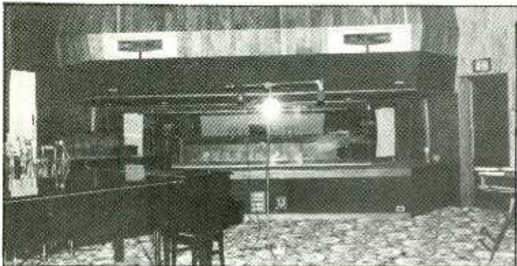
Westlake Studios control room with Harrison console, 3M 24-track and Studer 2-track and TMI monitors
