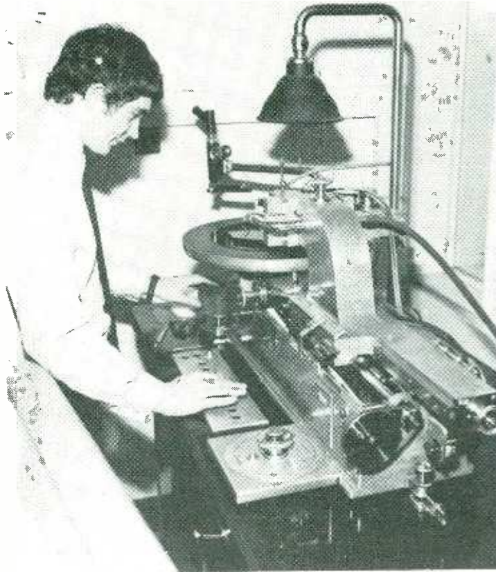
Above: Phil MacDonald cutting a master lacquer disc on a Scully lathe at Abbey Road (mid-sixties).
