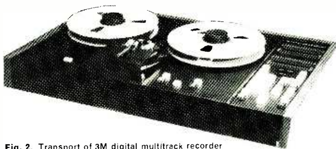
Fig. 2. Transport of 3M digital multitrack recorder
