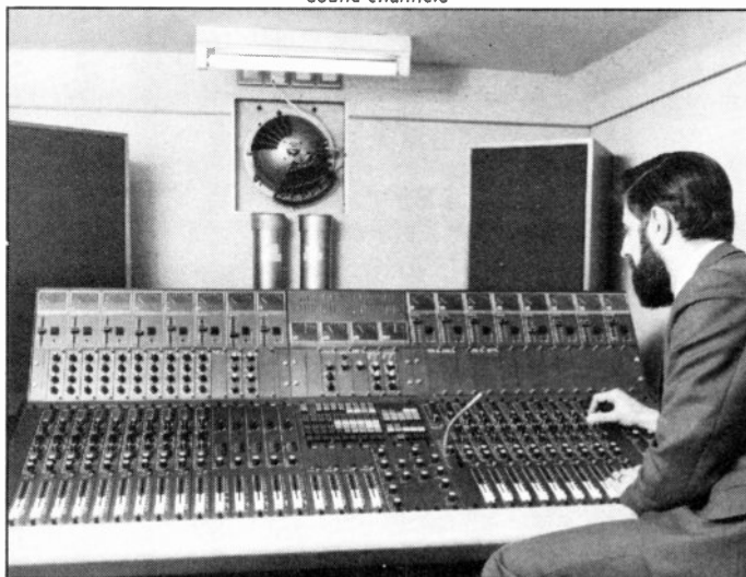
A special mixer installed in the IBA's mobile which includes five special surround sound channels
