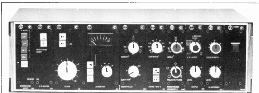
This photograph shows the current (production model) control unit required to operate the Soundfield microphone, as used by the BBC. The signal is fed from left to right via the following modules: the mic input module which takes the feeds direct from the mic head ('A-Format') after eq in the body of the mic, and offers individual mutes on the equalised capsule outputs plus a -20dB A-Format pad; the A-B matrix module which converts the A-Format signals to standard B-Format (X, W, Y, Z outputs corresponding to a front-facing figure-of-eight, omni, left-facing figure-eight and up-facing figure-eight respectively) and offers mic-inversion facilities; the B-Gain module which offers switched control of the B-Format level (+6, +14 and +20dB lift) and a rotary gain-control attenuator; the B-Format monitor module which offers individual PPM monitoring of the B channels plus overall levels; two Soundfield modification modules which control azimuth and elevation, and dominance; a mono/stereo/quadruple module which handles the coincidence angle and polar diagram settings; and two output modules, one equipped with Ambisonic decode/loudspeaker layout control and main output level control, the other controlling the stereo-output width and headphone-monitor level. To the far right of the unit is the power-supply module with power-on pushbutton.
