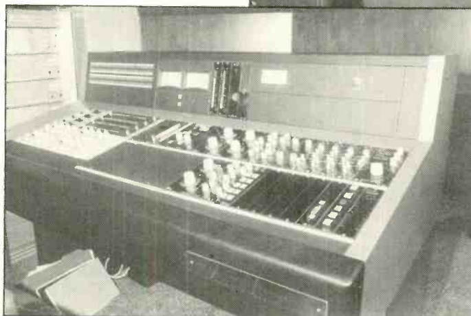
Tape 1 Studios: Above: Overall view of the new cutting room with JBL 4343 monitoring and Neumann SAL 74 drive amplifiers in evidence. Right: Neumann VMS-80 lathe Below: the customised Neumann SP79 cutting console
