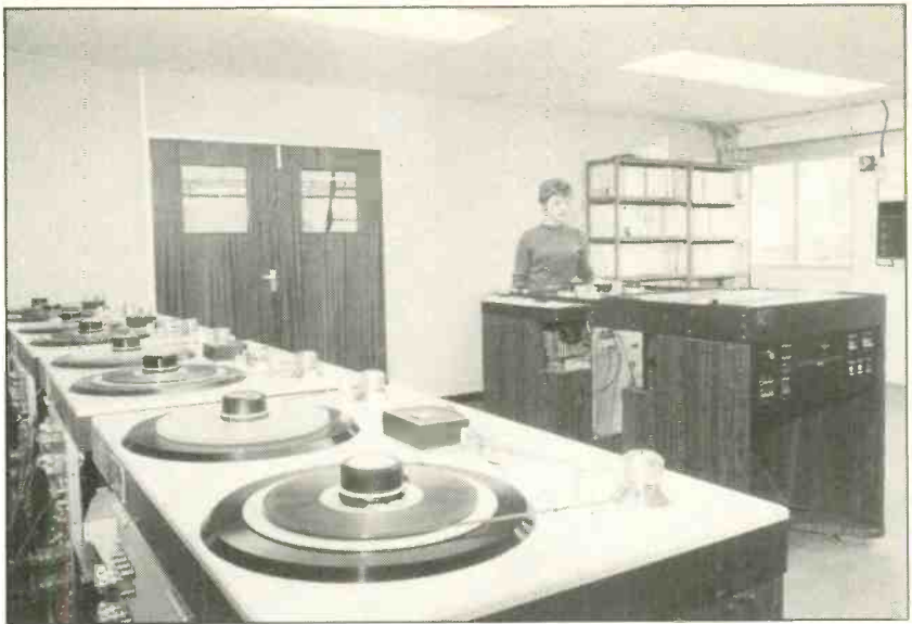
Tape duplicating room using Gauss 1" mastering playback machine with loop bin, and four tape duplicators
