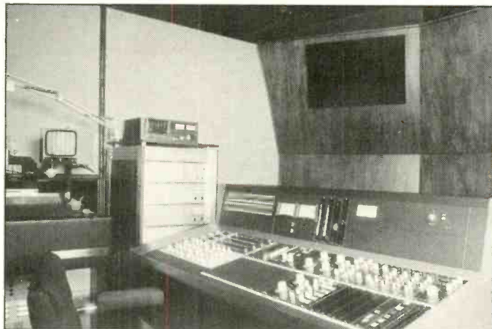
Tape 1 Studios: Above: Overall view of the new cutting room with JBL 4343 monitoring and Neumann SAL 74 drive amplifiers in evidence. Right: Neumann VMS-80 lathe Below: the customised Neumann SP79 cutting console
