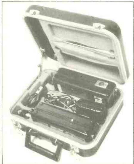
Carrying case with IE-30A realtime analyser, mains adaptor, IE-17A microprocessor analyser, probes and leads, and measuring mic in lid.
