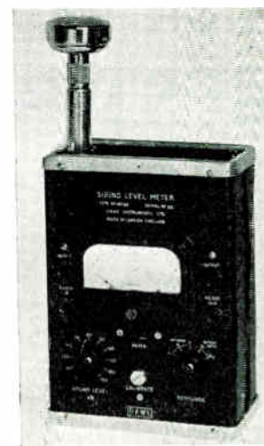
The sound level meter used by the author is the Dawe Instruments Type 1400E.
