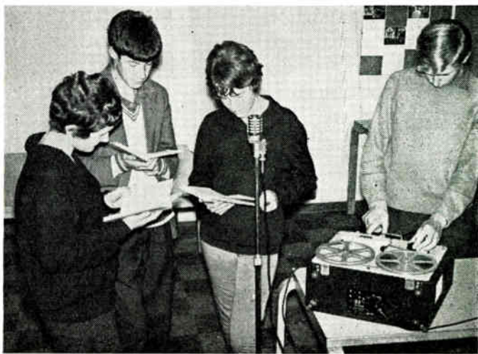
A play-reading run-through in progress. The microphone is a Reslo ribbon type, with "dead" angle towards the recorder.
