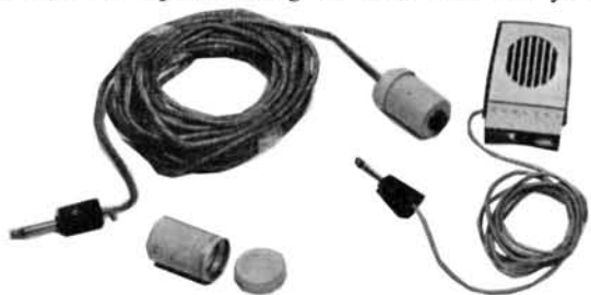
FIG. 3: Extending a microphone lead using a film container, jack socket and screened cable.
