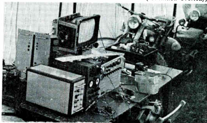
The photograph on the right shows the equipment required to operate one television camera. All this equipment was home-made by J. Tanner of Bristol.
