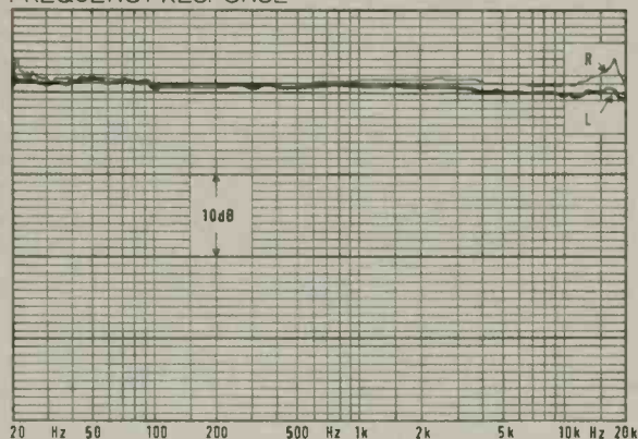
FIG. 1 STANTON 680EL FREQUENCY RESPONSE
