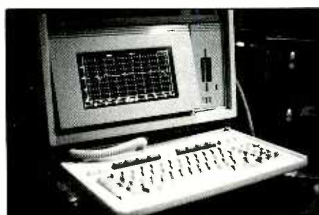
Hewlett Packard integral personal computer showing stored SIM trace
